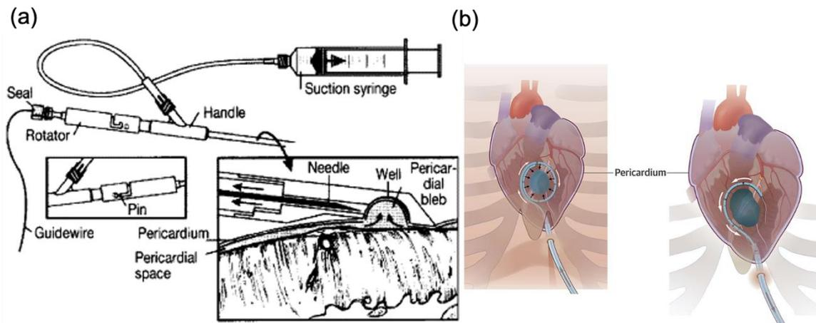
FIG 4. Schematic diagrams of the pericardial introducers (a) PerDUCER® [87] and (b) the loop catheter developed by Garcia *et al.*[48]
