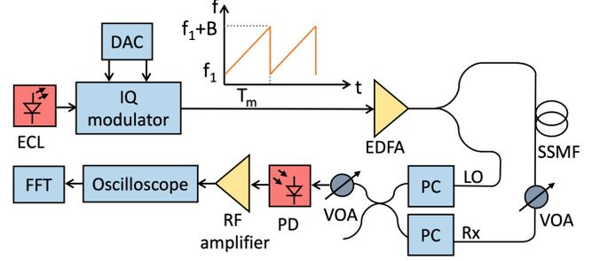
Fig. 2: System setup of single-photodiode based coherent LiDAR. ECL: external cavity laser; IQ: in-phase and quadrature; DAC: digital-to-analog converter; EDFA: Erbium-doped fiber amplifier; SSMF: standard single-mode fiber; VOA: variable optical attenuator; LO: local oscillator; Rx: received signal; PC: polarization controller; PD: photodiode; RF: radio frequency; FFT: fast Fourier transform.
