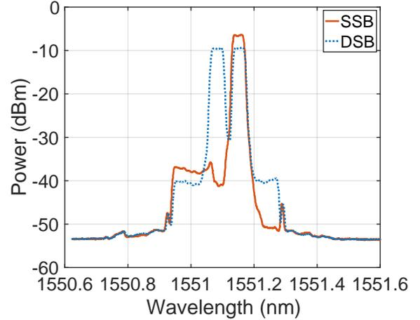
Fig. 3: Transmitted DSB and SSB signals (2 GHz guard band, 5 GHz chirp) measured by an optical spectrum analyzer at 0.01 nm resolution bandwidth.
