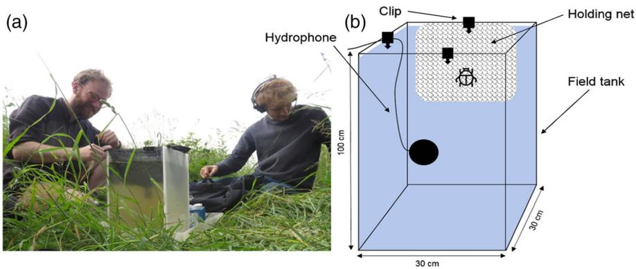
**FIGURE 2** Tank set-up used for recordings of the lesser-diving water beetle *Acilius sulcatus*, the cherrystone water beetle *Hyphydrus ovatus*, and the supertramp water beetle *Rhantus suturalis*: (a) field tank in situ; (b) field tank schematic
