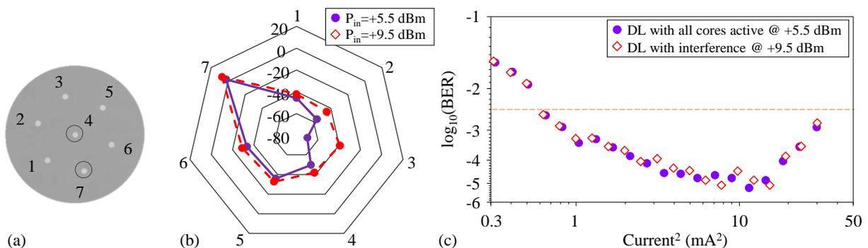
Figure 6. (a) Core distribution in the 7-core MCF. (b) Measured mean power (dBm) in each core of the 7-core MCF with an input power at core 7 of +5.5 dBm and +9.5 dBm. (c) BER performance vs. received squared photocurrent after 1-km MCF transmission for DL transmission (processed with 71 taps in the DD LMS equalization) with all cores active with +5.5 dBm and with +9.5 dBm interference.
