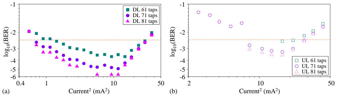
Figure 5. BER performance vs. received squared photocurrent after 1-km MCF transmission with the number of taps used in the DD LMS equalization (a) for DL and (b) for UL signal transmission.
