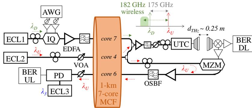
Figure 3. Experimental setup used for full-duplex transmission using the same wavelength for optical heterodyning at the DL and for UL transmission after 1-km of 7-core MCF and including a short-distance wireless link at 182 GHz.
