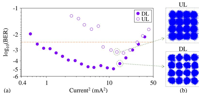
Figure 4. (a) BER performance vs. received squared photocurrent after 1-km MCF full-duplex transmission including DL and UL signals implementing wavelength re-use for DL heterodyning and UL transmission (both processed with 71 taps in the DD LMS equalization) and (b) received constellations for DL and UL.
