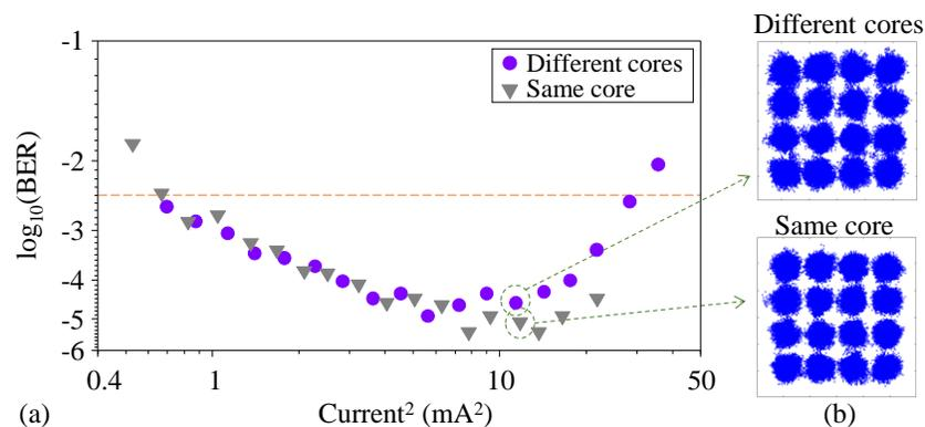
Figure 2. (a) BER performance vs. received squared photocurrent after 1-km MCF transmission over the same and over different cores (both processed with 71 taps in the DD LMS equalization) and (b) received constellations when both signals are transmitted over different cores (core 7 and 4) and over the same core (core 7).
