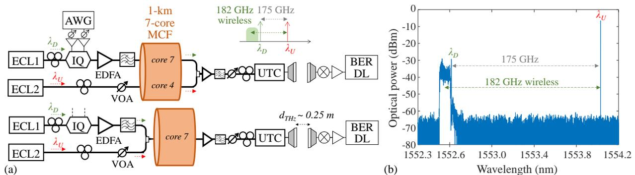
Figure 1. (a) Experimental setups developed for photonic THz generation using the same or different cores of a 1-km 7-core MCF link including wireless transmission at 182 GHz. (b) Measured optical spectrum at the UTC.
