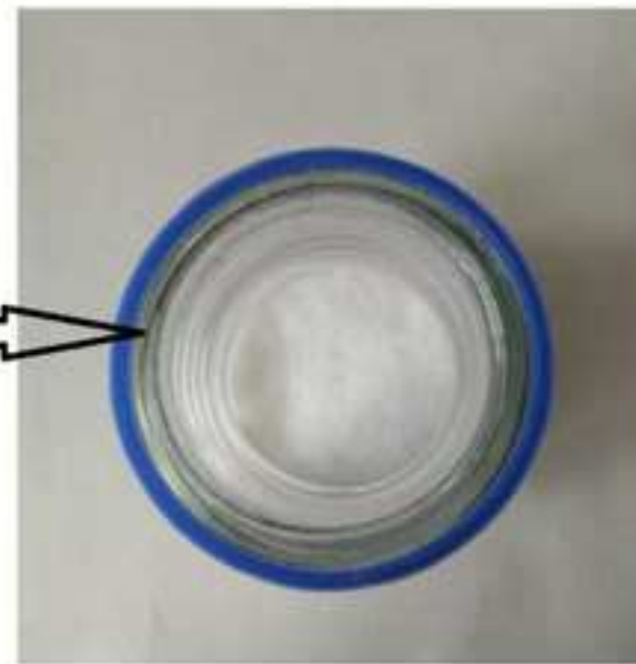
\text{Ho}_2\text{O}_3\text{-Yb}_2\text{O}_3/\text{SiO}_2 nanocomposite after calcination
