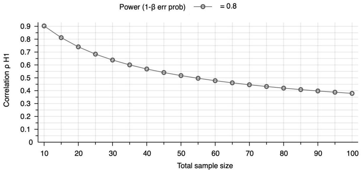
Figure A.1.1.1: Sensitivity curve plot of power (0.8) for desired alpha level (.002)
