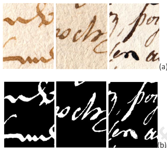
Figure 4. Comparison of (a) historical samples of different types of paper with iron gall ink and (b) the separation of pixels of ink from pixels of paper into binary images using k-means clustering over 420–870 nm.
