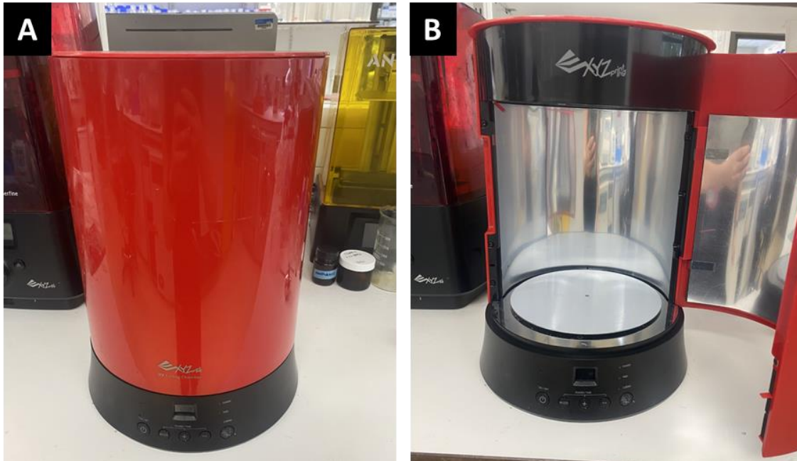
Figure 2-8: The XYZ Printing UV Chamber for the purpose of post curing the 3D printed models. Image (A) shows the chamber closed, with a solid red exterior to prevent any additional light emitting the chamber. Image (B) shows the chamber open, with the platform that the item is placed upon.
