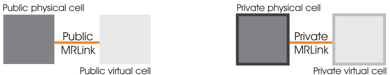
Figure 7: Public and private MRA Cells: Physical and virtual cells joined by Mixed Reality Links (Surrounding topology omitted). Cell boundaries as controlled by inhabitants determine level of privacy
