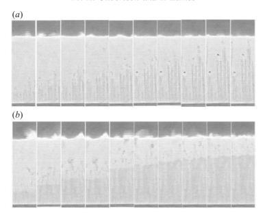
FIGURE 1. Time sequence showing the formation of segregation patterns by gas flowing through an initially homogeneous mixture of particles with equal proportions of  $45-90\,\mu m$  and  $250-425\,\mu m$  particles. The initial bed height is  $12.0\,c m$ . In (a) the gas flow rate is  $1.9\,c m\,s^{-1}$  and the time difference between each image is  $1.0\,s$ , and in (b) the gas flow rate is  $3.88\,c m\,s^{-1}$  and the time difference is  $2.0\,s$ .
