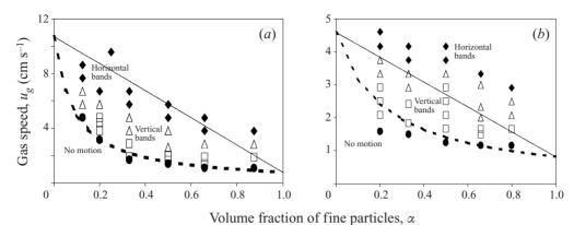
FIGURE 3. Phase diagrams for the mixtures of particles based on experimental observations. The different symbols correspond to the different structures seen: incipient motion ( $\bullet$ ); vertical bands ( $\square$ ); partial segregation ( $\triangle$ ); horizontal banding ( $\bullet$ ). (a) A mixture of 45–90 µm particles and 250–425 µm particles, and (b) a mixture of 45–90 µm particles and 190–212 µm particles.
