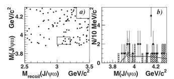
FIG. 4. (a)  $M_{\rm rec}(J/\psi\omega)$  vs  $M(J/\psi\omega)$ , and (b) projection onto  $M(J/\psi\omega)$ , showing the contributions from the  $\omega$  mass window (points with error bars) and sidebands [30 MeV/ $c^2$  <  $|M(\pi^+\pi^-\pi^0)-M_\omega|$  < 50 MeV/ $c^2$ , hatched histogram], the fit described in the text (solid line), and the 90% C.L. upper limit on the  $X(3940) \rightarrow J/\psi\omega$  contribution (dashed line).
