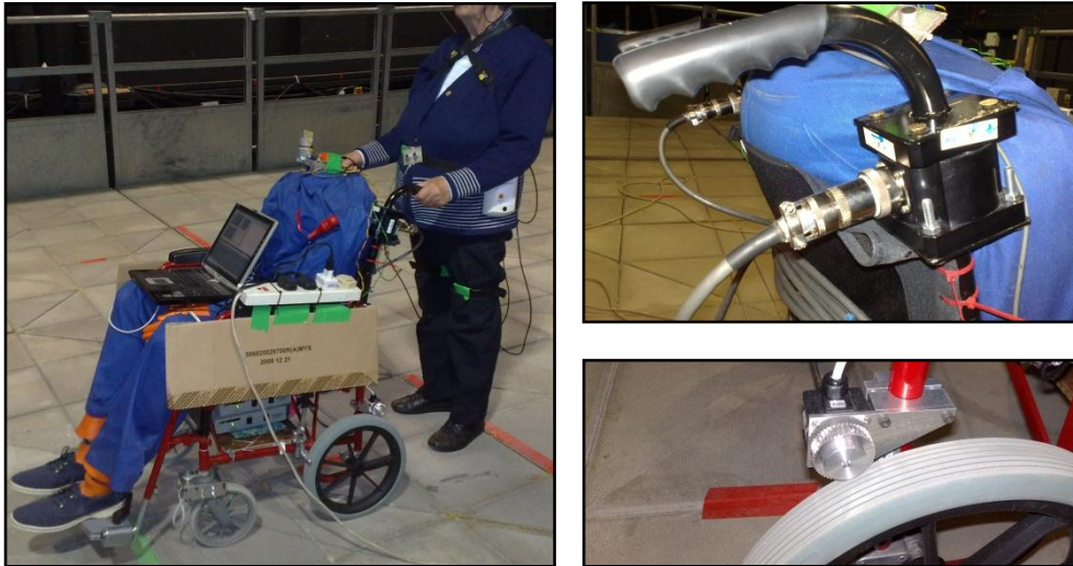
Figure 4-2: Attendant-propulsion wheelchair experiment system on left with detail of the force transducer (top right) and the rotary encoder used to measure the velocity (bottom right).
