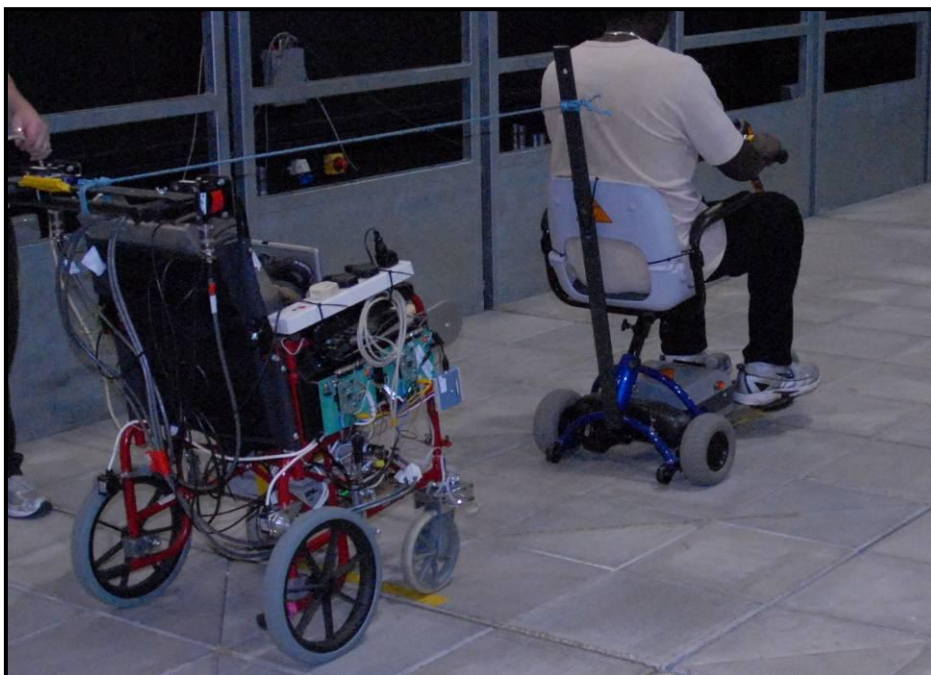
Figure A3-3: Experimental Procedure of pulling the wheelchair with the scooter. The wheelchair is attached to the scooter via a rope connected between the metal bars connecting the handles and a metal bar attached to the rear of the scooter.
