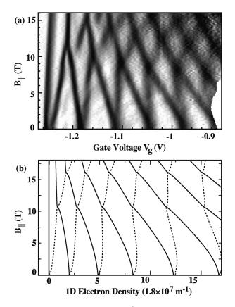
FIG. 3. (a) Gray-scale plot of  $dG/dV_g$  as a function of  $V_g$  and  $B_{\parallel}$  for sample B, showing the splitting of five 1D subbands. (b) Calculated Zeeman splitting with diamagnetic shift of the 1D subbands. The solid lines represent parallel spin and the dotted lines represent antiparallel spin.
