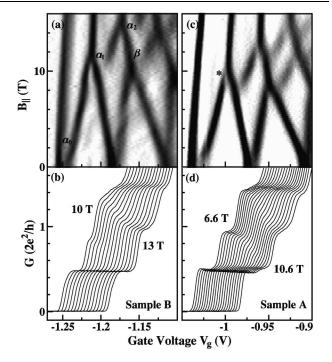
FIG. 2. (a) Gray-scale plot of transconductance,  $dG/dV_g$ , as a function of  $V_g$  and  $B_{\parallel}$  for sample B. (b)  $G(V_g)$  traces (offset horizontally) for  $B_{\parallel} = 10$  T to 13 T incremented by 0.2 T (sample B, different cooldown). (c) gray-scale plot as in (a), for sample A. (d)  $G(V_g)$  traces as in (b), for sample A.
