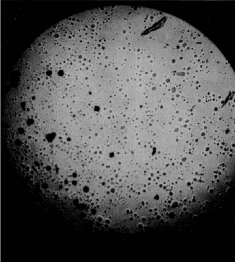
Fig. 2. Photograph of a Au-SiO<sub>x</sub>-Si device soon after forming, showing many small bubbles under the anode layer. Magn.  $\times 15$ .
