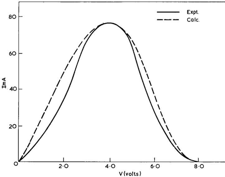
Fig. 7. The low-frequency or dc current-voltage behaviour calculated with the distribution of filament resistances shown in fig. 6b, compared with the experimental results of Simmons and Verderber<sup>10</sup>) in a formed Au-SiO<sub>x</sub>-Al device and after subtraction of the current before forming.
