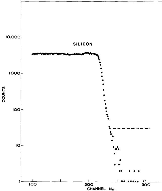
Fig. 5. The energy spectrum of 1.2 MeV protons back-scattered from a formed  $\text{SiO}_x$  film from which the gold anode had been removed. The dotted line indicates the level of counts to be expected (in that region of the spectrum) from  $10^{19}$  gold atoms per  $\text{cm}^3$  in the formed oxide.
