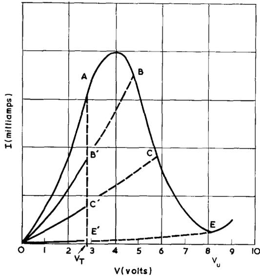
Fig. 3. Solid line: the dc or low-frequency current-voltage characteristic of a formed Au-SiO<sub>x</sub>-Al device, 400 Å thick. Broken lines: the dc (1 kHz) characteristics of the same structure [after Simmons and Verderber<sup>10</sup>].
