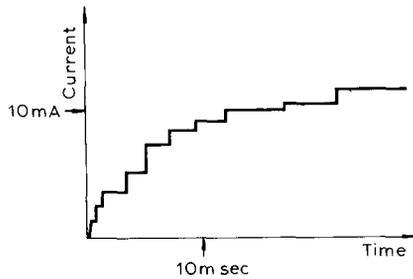
Fig. 4. Step-line increases of current as a function of time in the switching of a formed  $\text{SiO}_x$  film [after Greene et al.<sup>9</sup>].
