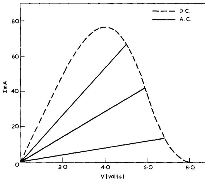
Fig. 8. The ac (1 kHz) current-voltage characteristic calculated in the filamentary model, assuming a simple triangular distribution of resistances (fig. 6b), and after the transient period has elapsed.
