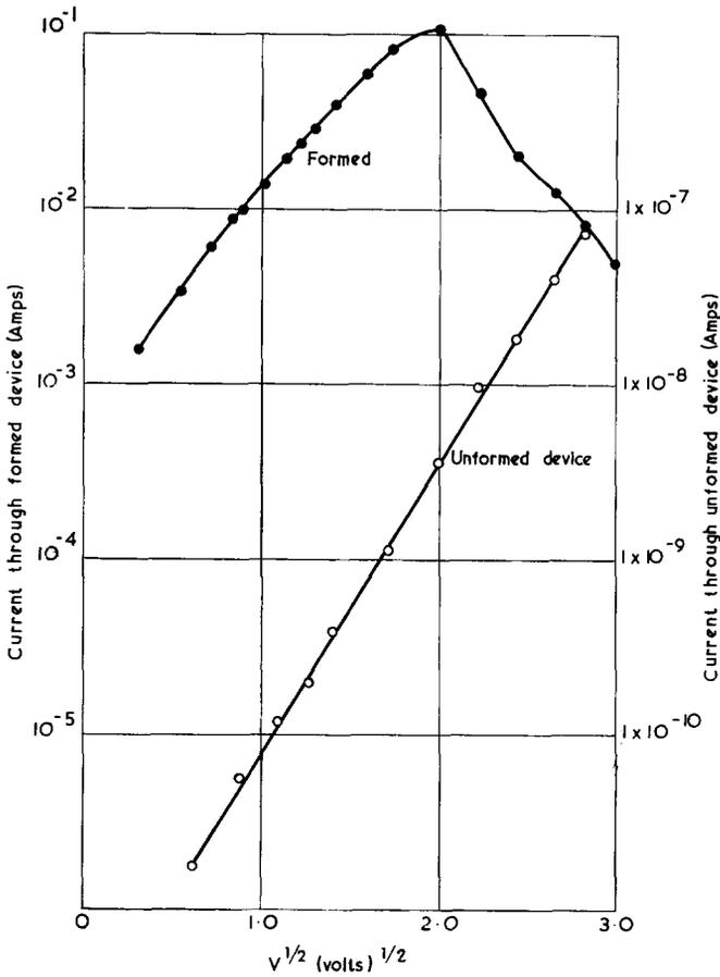
Fig. 1. Current-voltage characteristics of a gold-silicon monoxide-aluminium layer structure before and after forming, shown as a function of the square root of applied voltage. The oxide thickness was 400 Å [from Verderber et al.<sup>5</sup>].
