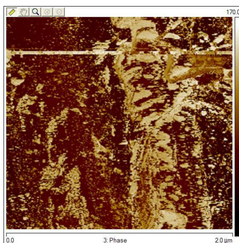
Figure 3.19. Tapping mode AFM images of the control ilomastat tablet. This indicates an inhomogeneous surface on the control tablet.
