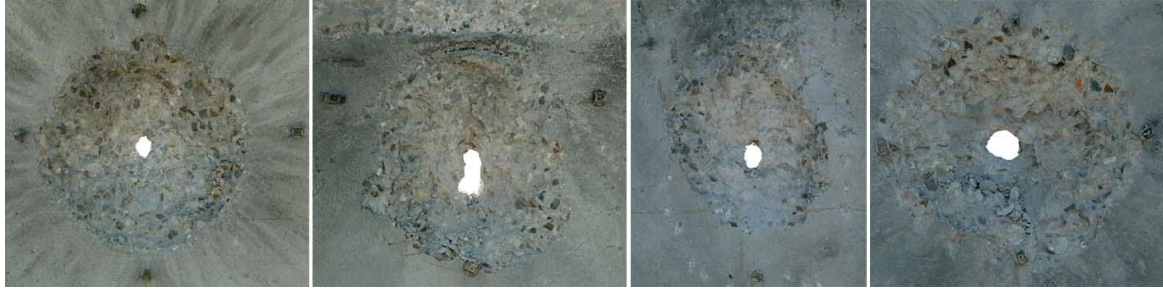
Figure 4.21: JC-EFP firings against Municipal target, (left to right) 1CD at 90°, 1CD at 45°, 3CD at 45° and 3CD at 90°
