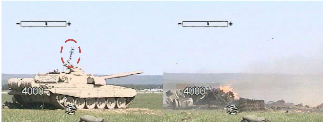
Figure 1.7: Javelin missile in terminal dive phase (circled left) and destroyed T72 following detonation of stored ammunition and propellant (right)
