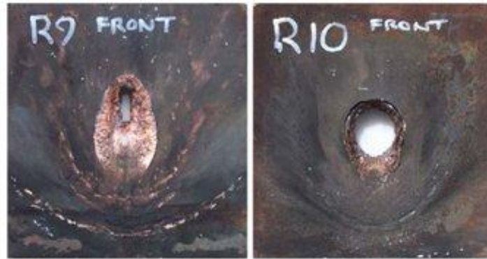
Figure 4.9: Medium armour RHA target perforation 1CD stand-off 45° obliquity, JC-EFP (left) and CSSJ (right)
