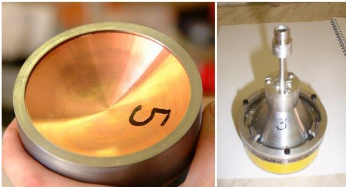
Figure 4.1: CSSJ liner profile (left) and built - ready to fire (right)
