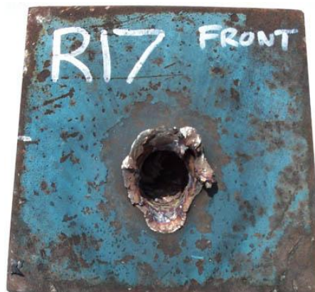
Figure 4.13: Damage sustained by MBT RHA plate at 45° obliquity
