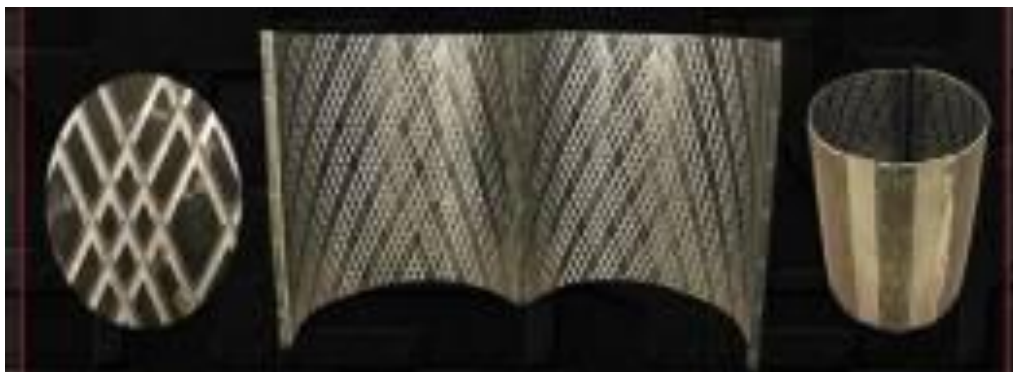
Figure 1.11: Hellfire II K variant Tantalum fragmentation overwrap (image courtesy of AMRDEC)
