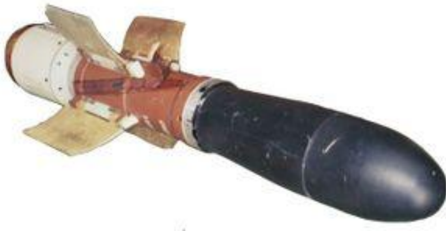
Figure 1.4: Milan missile with fins deployed (image courtesy of Jane's Information Systems)
