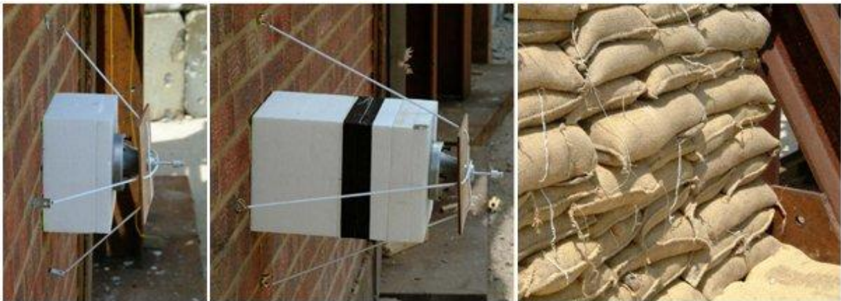
Figure 4.16: CSSJ warhead at 1CD stand-off / 90° obliquity (left) 3CD stand-off / 90° obliquity (middle) and sandbag fortification to the rear of the Fortified urban target
