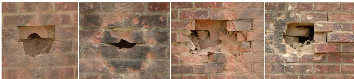
Figure 4.18: CSSJ firings against Fortified urban target, (left to right) 1CD at 90°, 3CD at 90°, 1CD at 45° and 3CD at 45°
