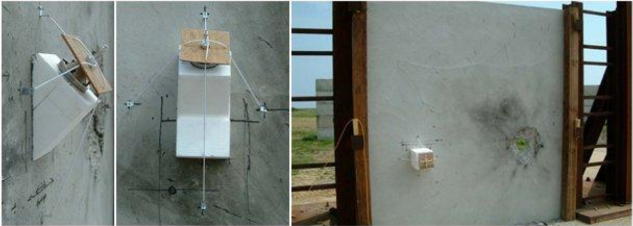
Figure 4.17: CSSJ warhead at 1CD stand-off / 45° obliquity (left) 3CD stand-off / 45° obliquity (middle) and front view of the 3m x 3m Municipal target
