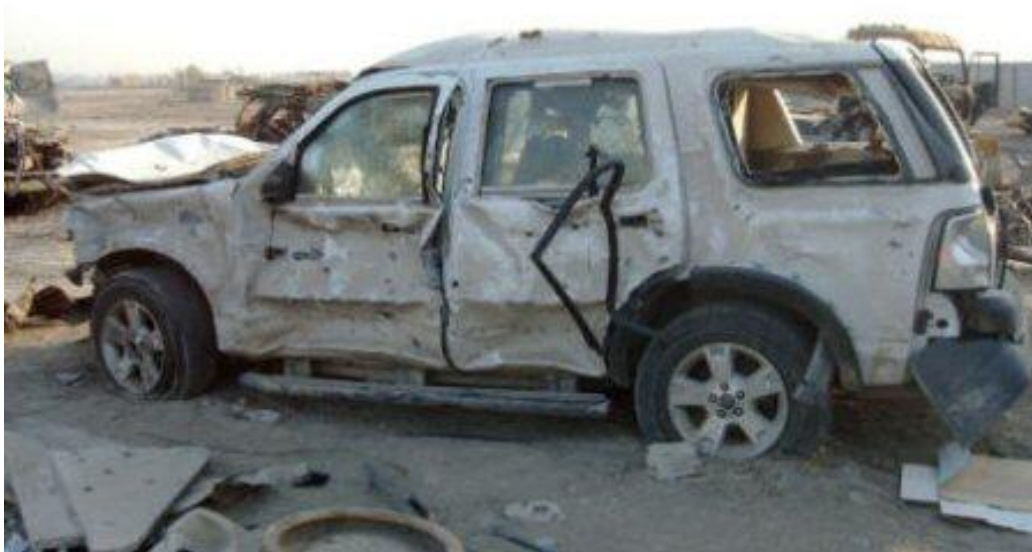
Figure 1.9: Blast damage to a First Defense International Group's armoured Ford® Expedition® 8 (image courtesy of Newsbusters)
