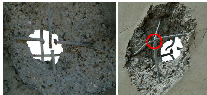
Figure 4.20: CSSJ firing against reinforcing bars of Municipal target, 1CD at 90°
