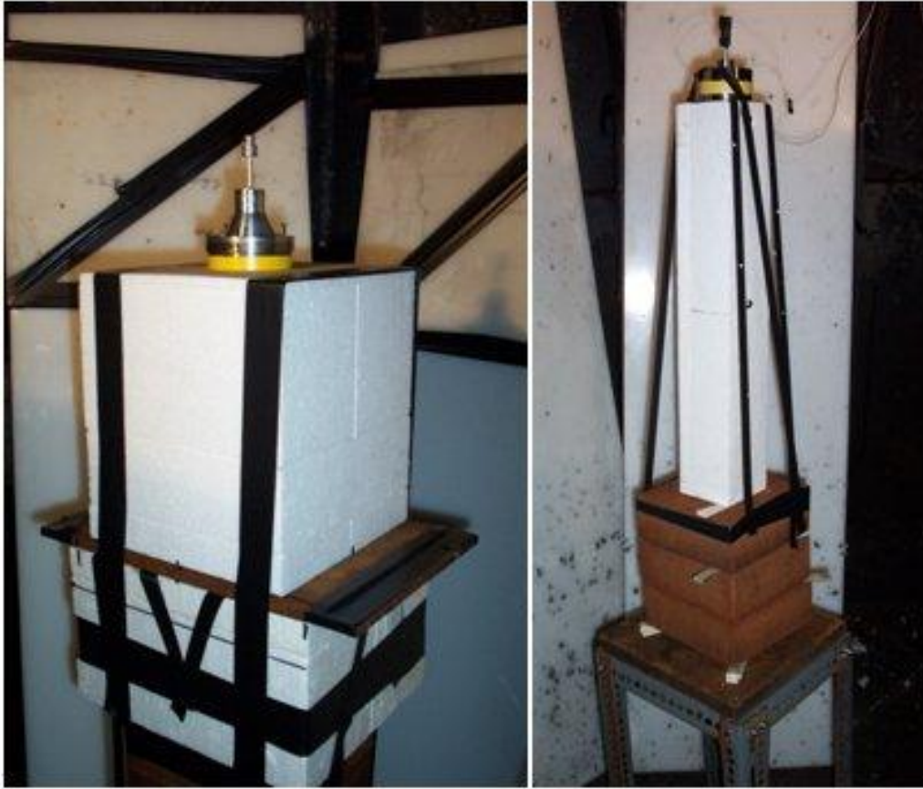
Figure 4.7: The CSSJ (left) and the JC-EFP(right) prepared for firing
