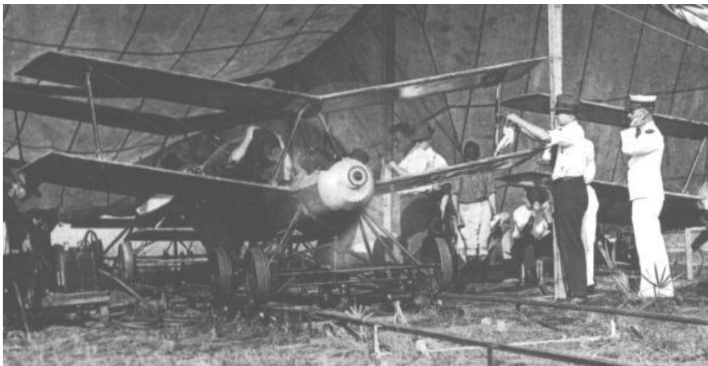
Figure 2.17: The Kettering Bug being prepared for a test flight (image courtesy of US Air Force museum)
