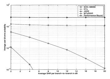
Fig. 8. Average error probabilities for a three-user MIMO system with six BS antennas, two antennas/MS, and  $(K_1, K_2, K_3) = (2, 2, 2)$ .
