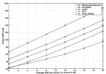
Fig. 5. Simulation results for a three-user MIMO system with six BS antennas, six antennas/MS, and  $(K_1, K_2, K_3) = (2, 2, 2)$ .
