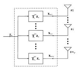
Fig. 2. System configuration of space–time preprocessing network for the mth user.
