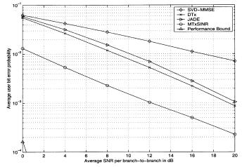
Fig. 6. Average error probabilities for a three-user MIMO system with six BS antennas, six antennas/MS, and  $(K_1, K_2, K_3) = (2, 2, 2)$ .
