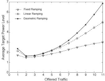
Fig. 5. Average target power level of preamble transmission.
