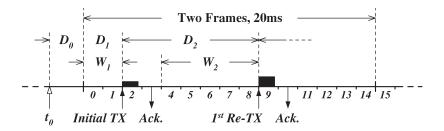
Fig. 2. Access mechanism of preamble transmission.
