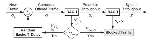
Fig. 1. Flow diagram of random access request.
