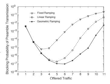
Fig. 6. Blocking probability of preamble transmission.
