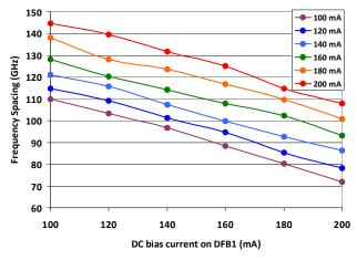
Fig. 2. Dependence of the frequency spacing between DFB1 and DFB2 wavelengths as the DFB1 current is varied at various fixed values of DFB2 current.
