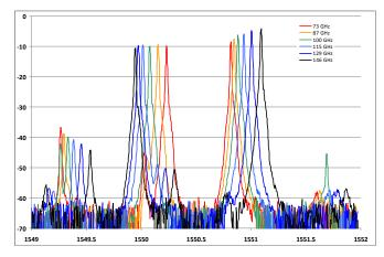
Fig. 3. Optical spectra obtained for various combinations of  $I_{DFB1}$  and  $I_{DFB2}$  currents generating increasing frequency spacing.
