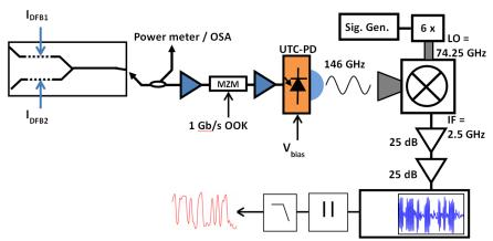
Fig. 4. Schematic diagram for the experimental 146-GHz wireless transmission system.
