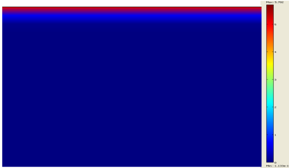
Figure 7. 10 Cross-sectional concentration profile of CO 2 in the liquid side at a length of ( z/\delta_L = 77.5 ) with the use of staggered herringbones. PTFE porosity \approx 65\text{-}70\% , \delta_G = 850 \mu\text{m} , \delta_L = 200 \mu\text{m} , NaOH 2M, Y_{\text{CO}_2}/Y_{\text{NaOH}} = 96.4 , Pe \sim 10^3 .
