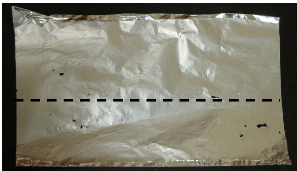
Figure 8. 3 Aluminium foil used to determine the distribution of cavitation intensity in the ultrasonic cleaner.
