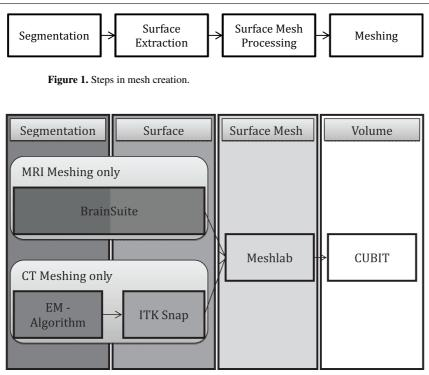
Figure 2. Software used in the four main steps of MRI and CT meshing.
