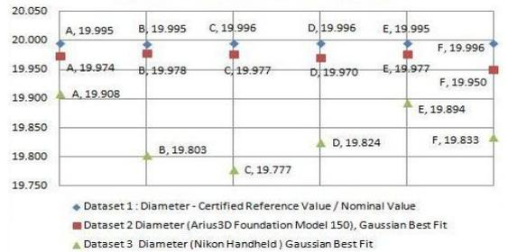
Figure 14 Sphere diameter values, absolute values in [mm]
