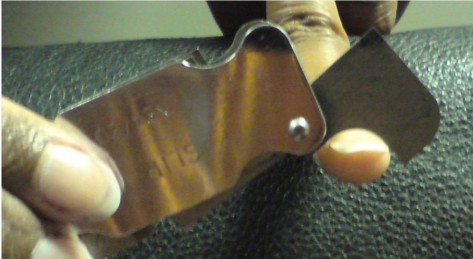
Figure 3: The measurement of transverse nail curvature using a radius gauge
