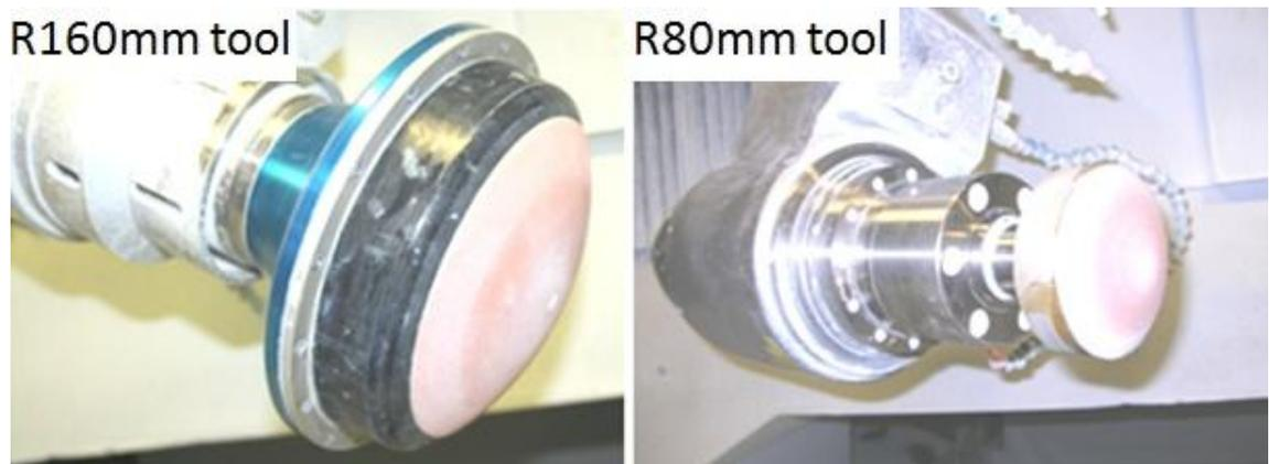
**Figure 6.5** The tools for the experiment, where on the left is the R160mm tool, and on the right is the R80mm tool (picture by author, 2011)
