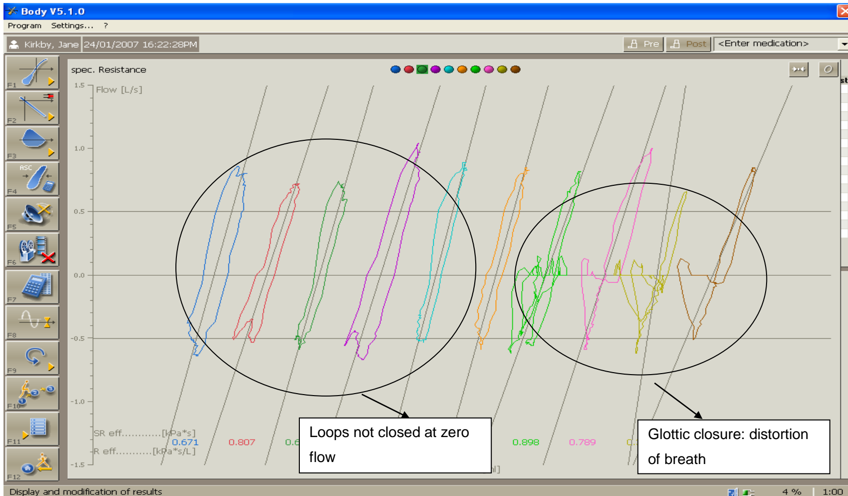
Figure 2-16: Example of sRaw data which failed QC criteria
