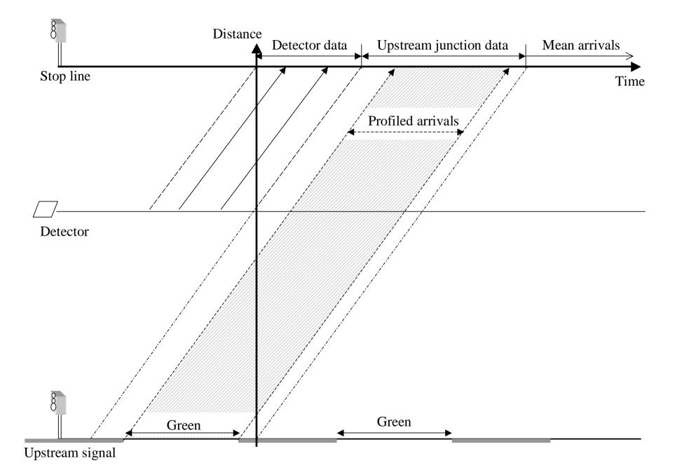
Figure 3: Sources of data for feedforward control of traffic signals
