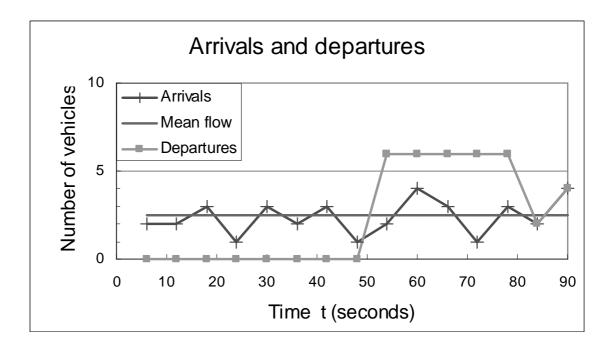
Figure 2: arrival and departure profiles during a signal cycle
