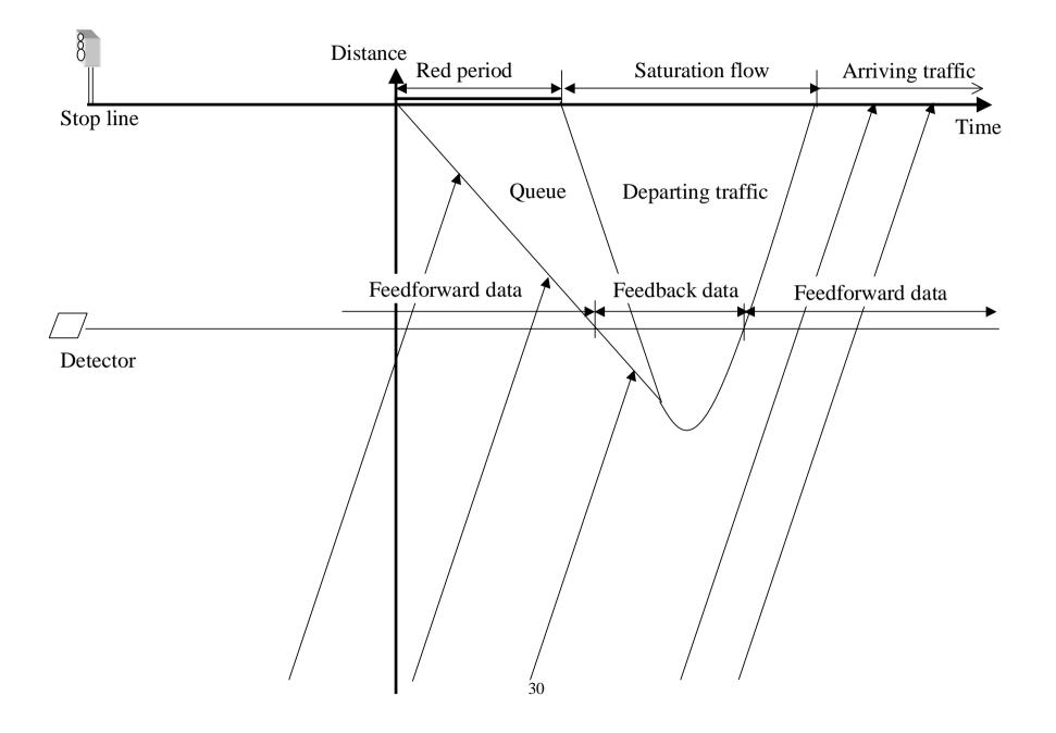
Figure 4: Nature of data from an upstream detector.
