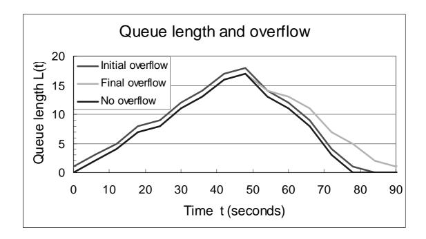
Figure 1: Queue length profiles illustrating various overflow possibilities
