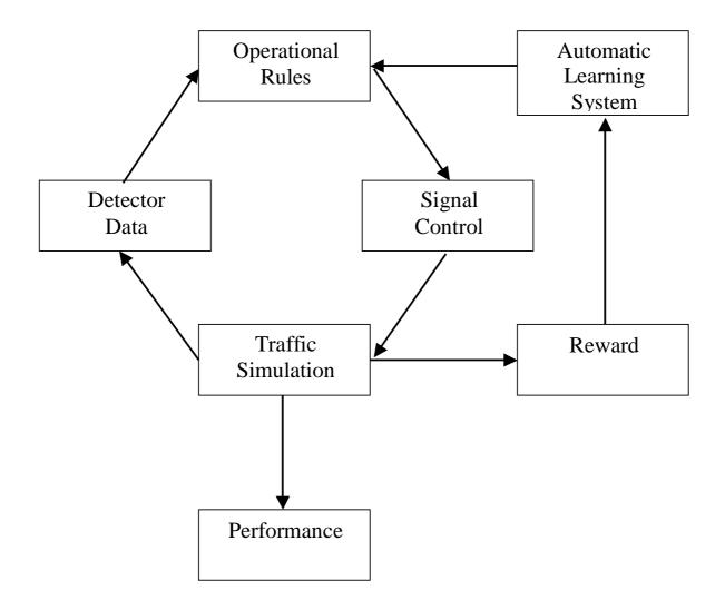
Figure 5: Structure of an automated learning system for traffic signal control
