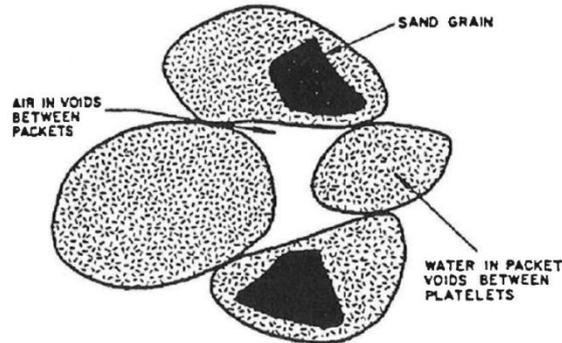
Figure 3: Model of unsaturated soil (Brackley, 1975)
