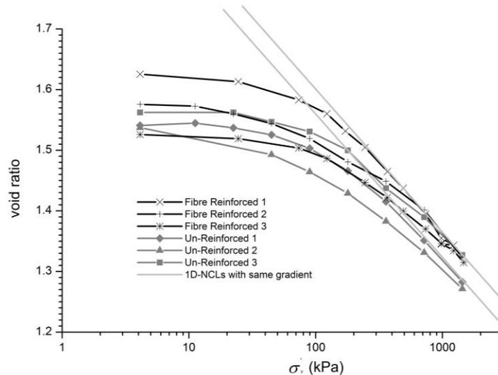
Figure 5: One-dimensional compression of fibre-reinforced and unreinforced clay samples
