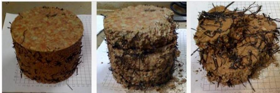
Photo3: Extruding fibres from sample
