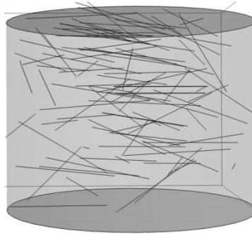
Figure 8: 3D orientation of the fibres on a dissected sample
