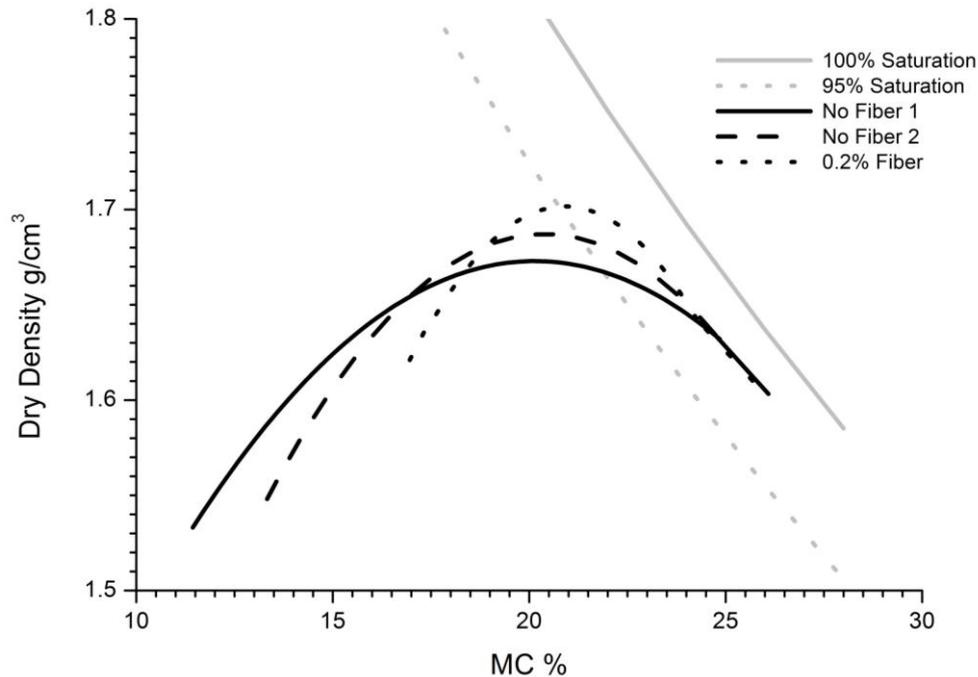
Figure 2: Compaction Curves of reinforced and non-reinforced samples
