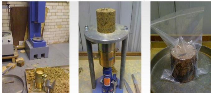
Photo 2: Reinforced sample compaction procedure
