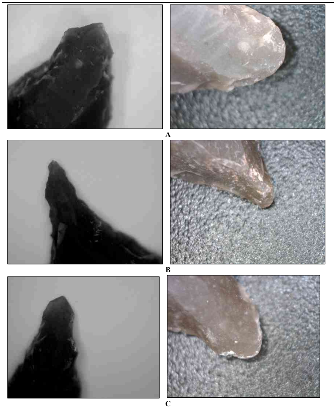
Figure 2.3.16. Photographs of experimental flint drills or microdrills before (left) and after heavy use (right): A) drill used on schist (Mohs 4-5); B) microdrill used on limestone (Mohs 2-3); and C) drill used with abrasive on hard marble (Mohs 5)
