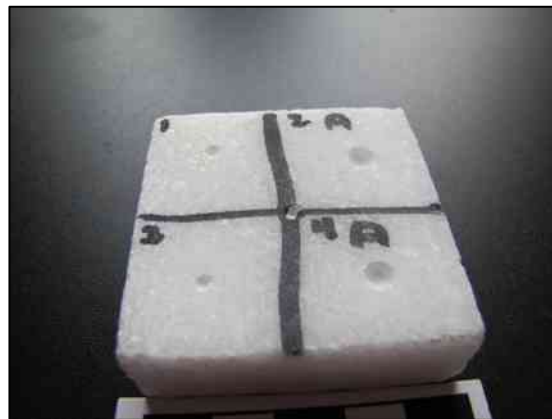
Figure 2.3.15. Experimental marble block with incomplete perforations (left side without abrasive, right side with abrasive) made using a mechanical drill within the same 2 minute set time
