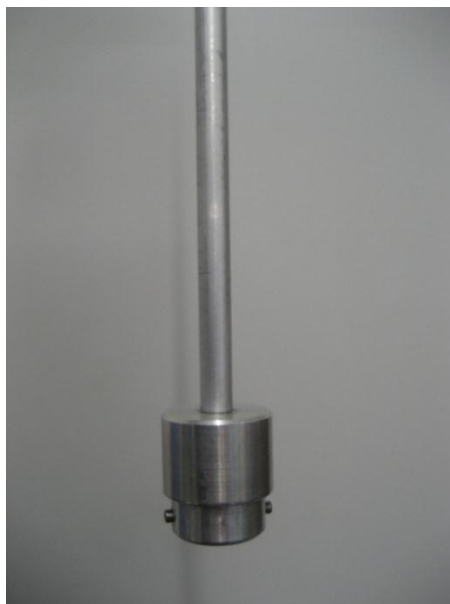
FIGURE 3.18. : Special rod used to lift and lower the new ampoules in the calorimetric chambers.
