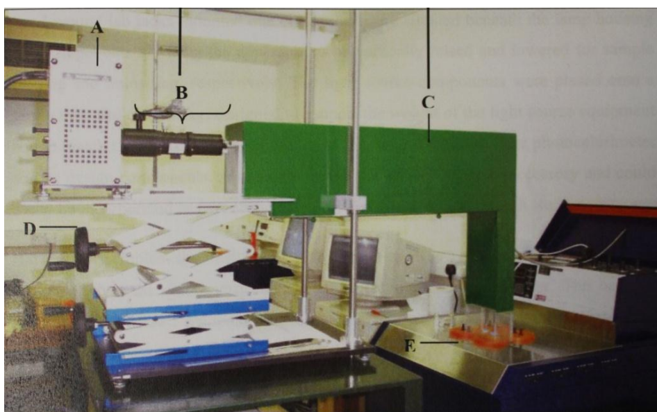
FIGURE 1.7. : Morris' photocalorimeter (taken from (4)). A: lamp housing fitted with a 300 W Xe arc lamp; B: filter/lens assembly; C: plastic shrouding surrounding light guide; D: hand-wound lab jacks; E: optical cables lowered into TAM calorimetric unit. Note: monochromator not shown.
