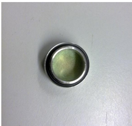
FIGURE 5.15. : Sample of 2-NB after photodegradation in the photo-MCDSC
