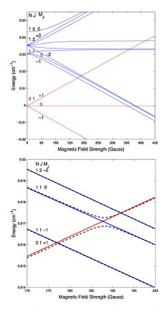
FIG. 1 (color online). Energy levels of KRb as a function of magnetic field *B*. The upper panel shows an overview, with each zero-field level [labeled by (N, J)] splitting into 2J + 1 components as a function of magnetic field. The lower panel shows how two levels of different parity cross  $(M_J = 0 \text{ and } +1)$  in the absence of an electric field (solid lines) but avoid one another in the presence of a 5 kV/cm electric field (dashed lines).
