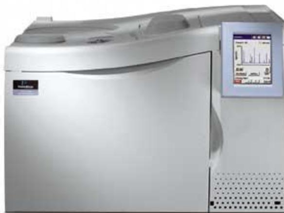
**Figure 5.1:** Perkin Elmer Clarus 500 GC with WCOT fused silica 60m × 0.25mm internal diameter (CP7818) column. Temperature program: starting at 80°C for 5 minutes then ramping at 10°C/min to 250°C for 8 minutes.
