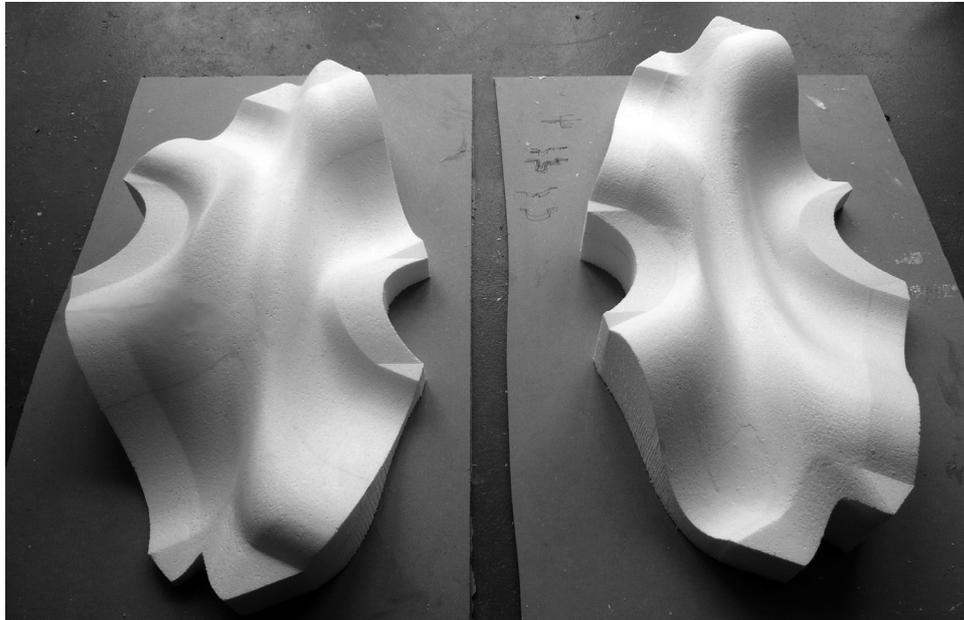
**Fig. 6i** the two beds for flip milling and for fibreglass mould
