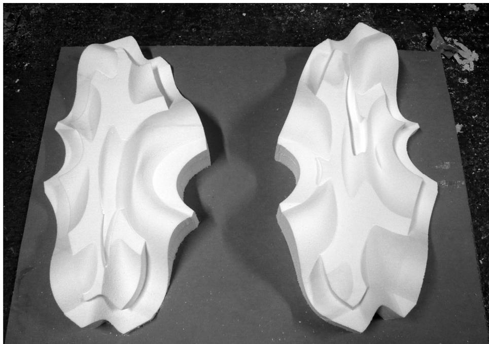
**Fig. 6j** the two beds on which the positive tile is being milled in 2 horizontal laminations
