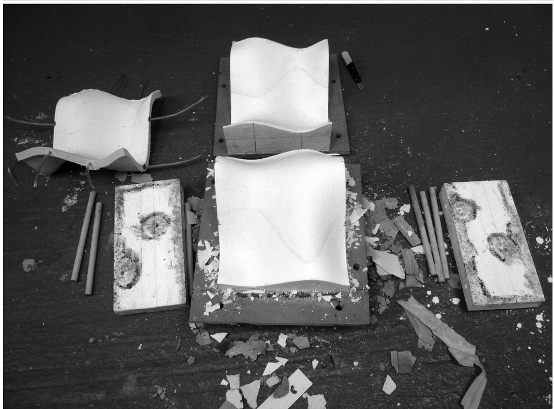
**F10.** Formwork before and after casting
