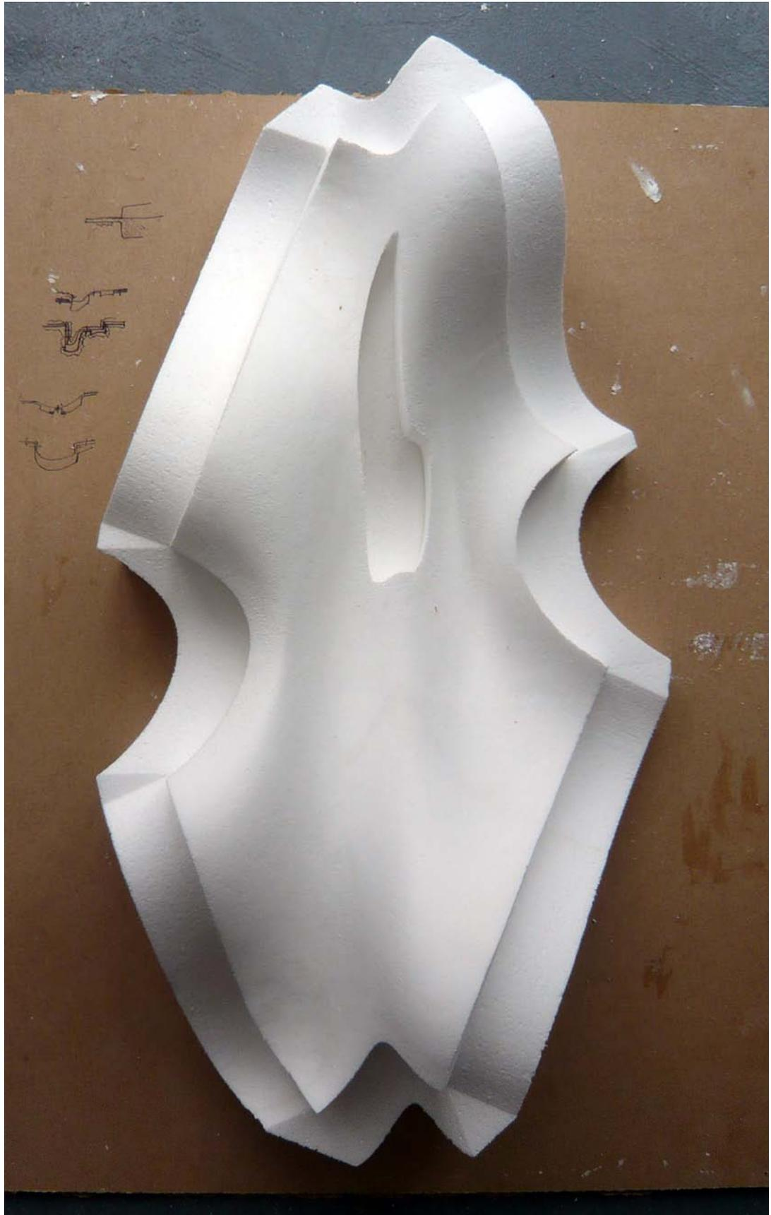
**F8.** NURBS tile from quasi cylinder; one bed and positive tile for fibreglass mould
