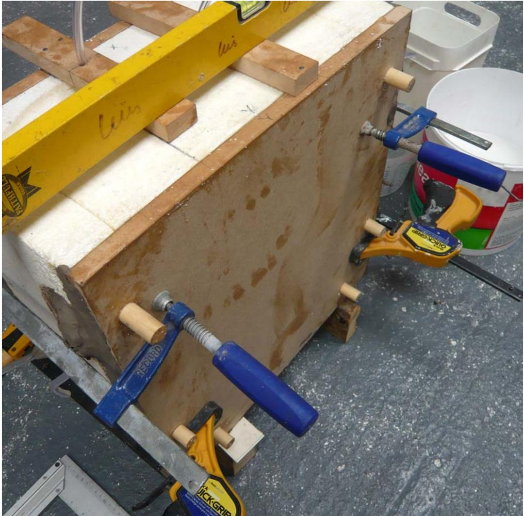
F11. Ready formwork for casting
