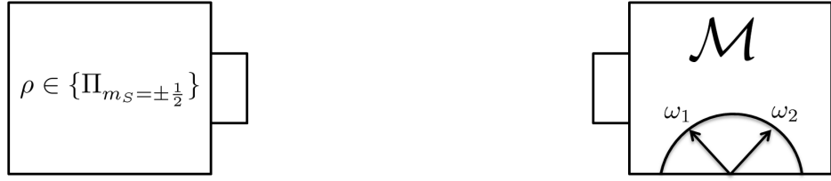
Figure 2.2: A simplified depiction of the Stern Gerlach experiment. A preparation device can switch between preparing a spin one-half particle with m_S = +\frac{1}{2} and m_S = -\frac{1}{2} . If the measurement is sharp, then an event \omega_1 will determine that the particle was of spin m_S = +\frac{1}{2} and conversely for the other event.
