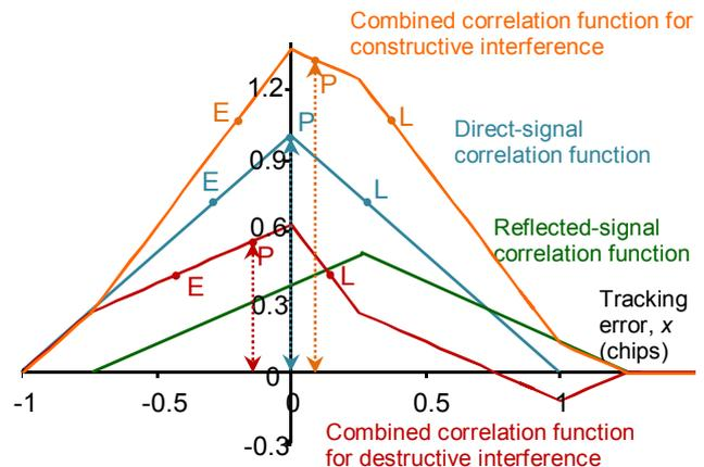
Figure 2: Effect of constructive and destructive multipath interference on size of prompt (P) correlator output (path delay = 0.25 chips; relative amplitude of reflected signal = 0.5; adapted from [7])
