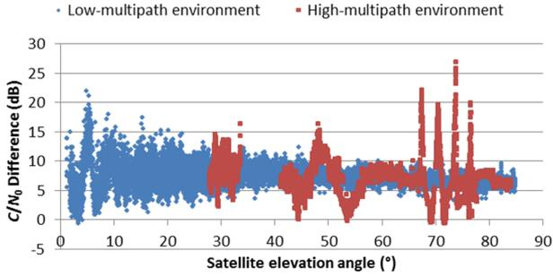
Figure 4: Comparison of low-multipath and high-multipath L1-L2  $C/N_0$  differences for GPS PRN 25
