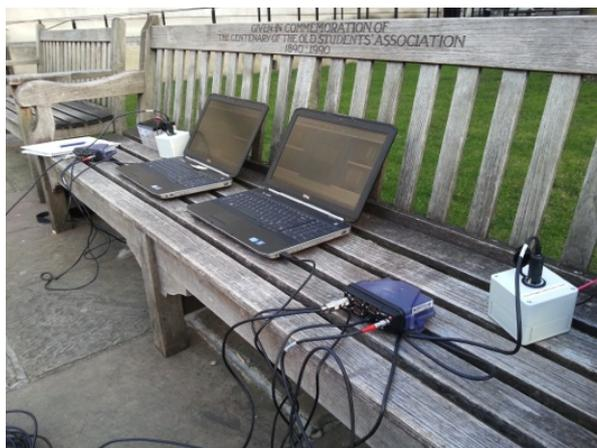
Figure 13: Two Novatel Flexpak 6 OEM628 GNSS receivers and logging PCs.
