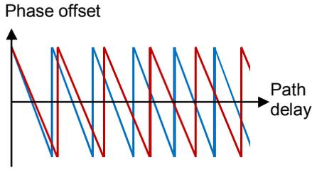
Figure 3: Phase offset of the reflected signal with respect to the direct signal on two different frequencies as a function of the path delay
