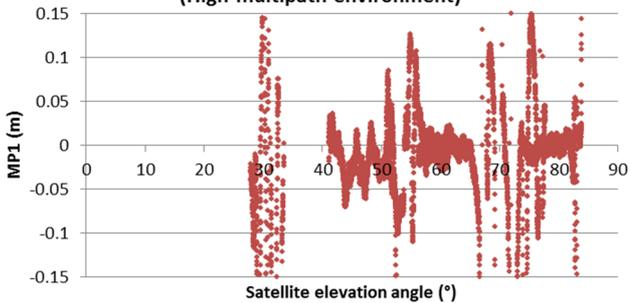
Figure 6: MP1 parameter for GPS PRN 25 in a high-multipath environment
