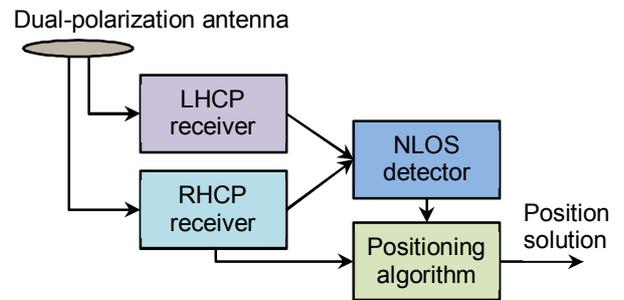
Figure 11: Dual-polarization NLOS detection method
