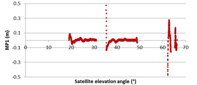
Figure 8: MP1 parameter for GLONASS R12 in a high-multipath environment
