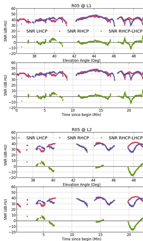
Figure 14: RHCP, LHCP and differenced  $C/N_0$  for GLONASS satellite R05 at Gower Place test site.
