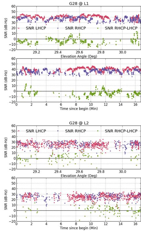
Figure 18: RHCP, LHCP and differenced  $C/N_0$  for GPS satellite G28 at Starbucks, Euston Square test site.
