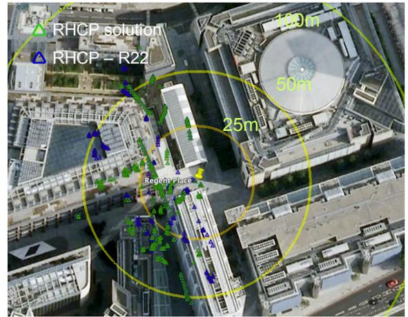
Figure 22: Position solutions with and without GLONASS satellite R22 at Regent Place test site (Background image © 2013 Bluesky).
