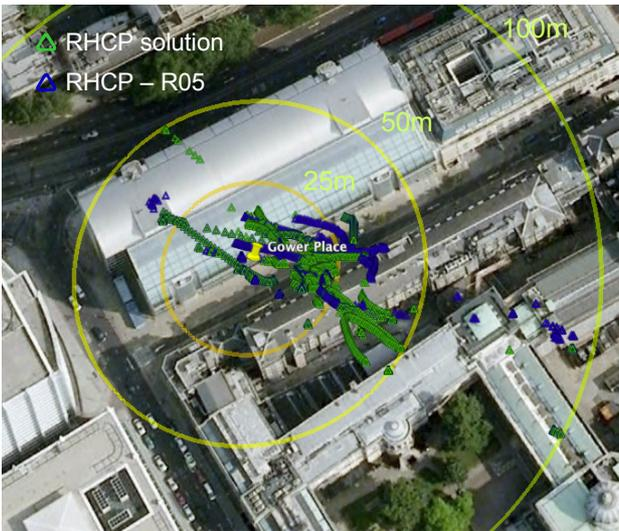
Figure 19: Position solutions with and without GLONASS satellite R05 at Gower Place test site (Background image © 2013 Bluesky).
