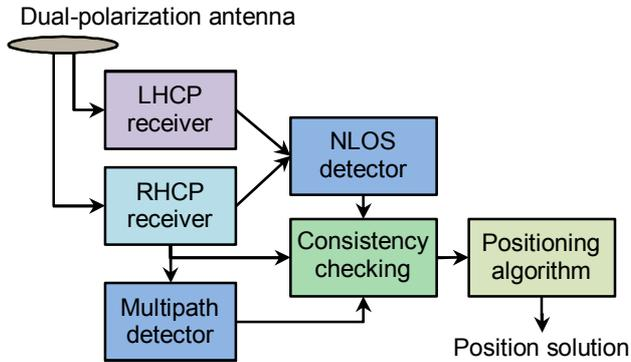
Figure 24: NLOS and multipath mitigation portfolio for professional applications (The multipath detector incorporates both early-late correlator comparison and multi-frequency  $C/N_0$  comparison)
