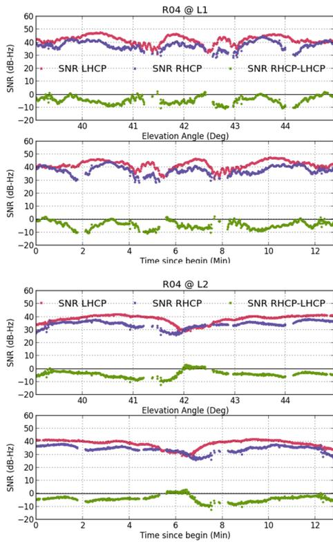
Figure 15: RHCP, LHCP and differenced  $C/N_0$  for GLONASS satellite R04 at Stephenson Way test site.
