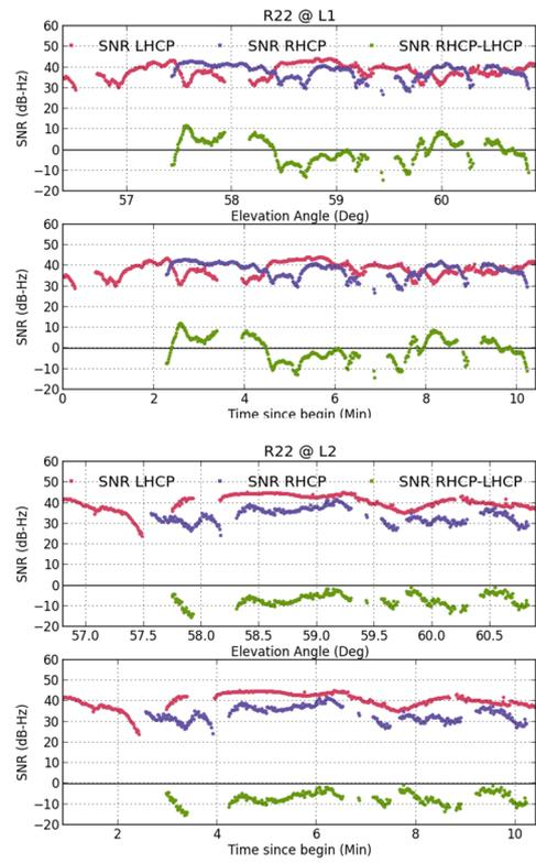
Figure 17: RHCP, LHCP and differenced  $C/N_0$  for GLONASS satellite R22 at Regent Place test site.
