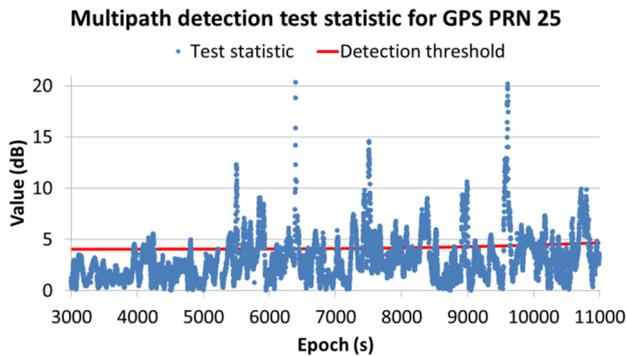
Figure 9: Three-frequency multipath detection test statistic and detection threshold for GPS PRN 25 at the urban test site near Birkbeck College, London
