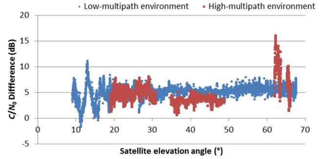
Figure 7: Comparison of low-multipath and high-multipath L1-L2  $C/N_0$  differences for GLONASS R12
