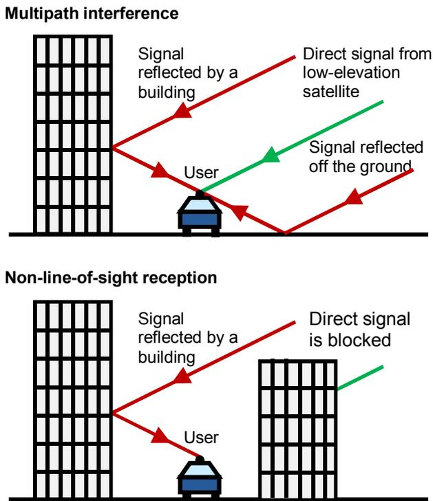
Figure 1: Multipath interference and NLOS reception
