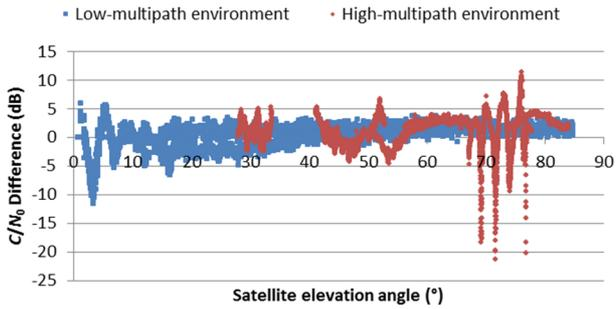
Figure 5: Comparison of low-multipath and high-multipath L1-L5  $C/N_0$  differences for GPS PRN 25
