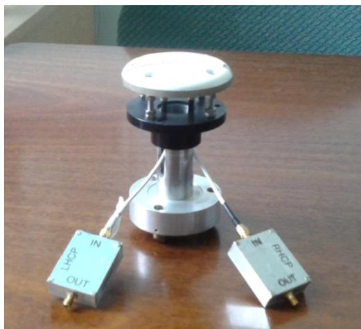
Figure 12: Antcom 3G1215RL-P-XS-1 dual-polarization antenna, mounting and amplifiers.
