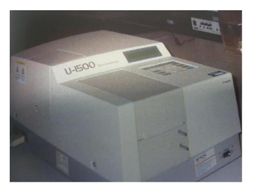
Figure 26: Spectrophotometer (model U-1500; HITACHI. WOKINGHAM, UK).
