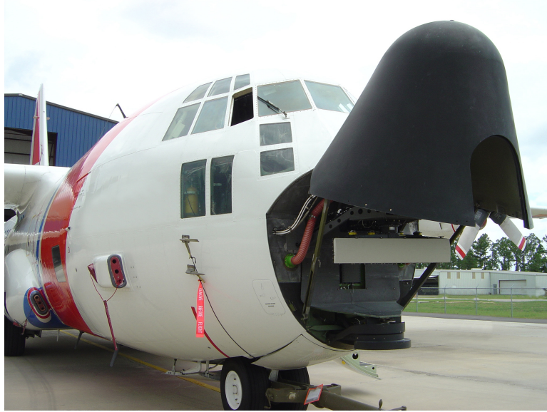
Figure 1.4: Seaspray 7500E radar mounted in U.S Coast Guard HC-130 Hercules
