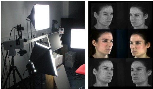
Figure 1. Dynamic 3D Stereo Camera used for data collection. Six cameras combine to provide 3D reconstructions of the face, with a recording rate of 60 FPS.
