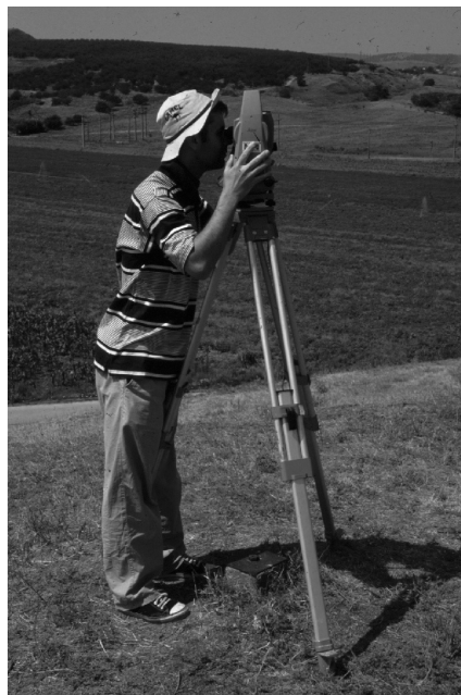
Figure 1. Total station being used for contour survey on the Roman site of Noviodunum, Romania (courtesy of Kris Lockyear)
