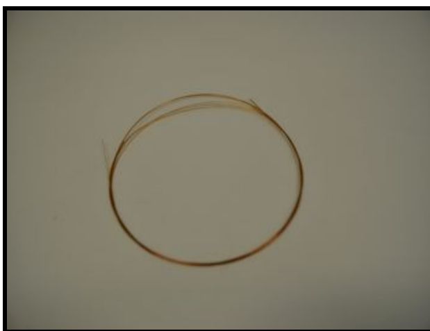
Figure 4.1: Fused silica capillary for the construction of the immobilised enzyme capillary reactor.
