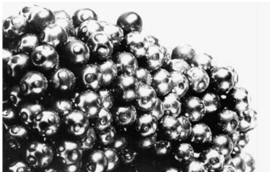
Figure 11. Part of a random packing of steel balls taken from a paint-fixed model.
