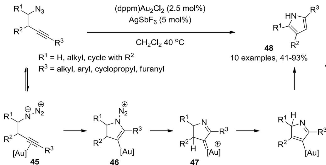
Scheme 26: Intramolecular acetylenic Schmidt reaction <sup>47</sup>
