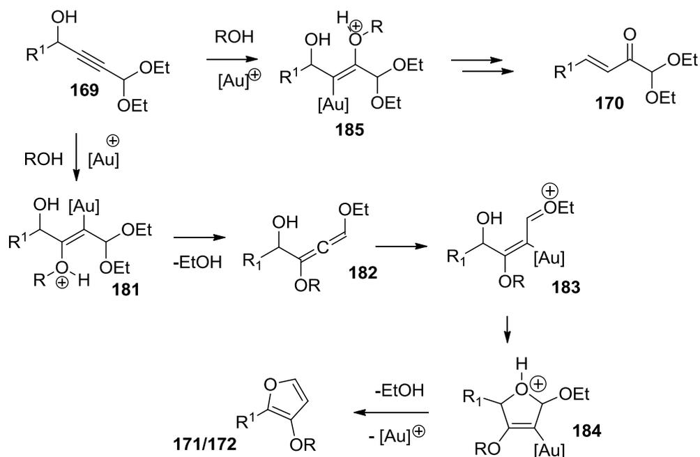
Scheme 104: Possible mechanism for the Au-catalysed furan synthesis.
