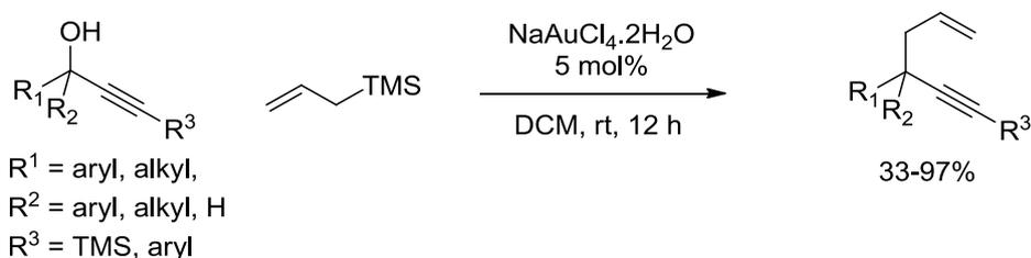
Scheme 43: Au catalysed propargylic substitution<sup>81</sup>
