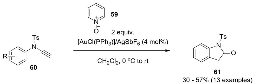
Scheme 30: Au-catalysed synthesis of oxindoles<sup>54</sup>
