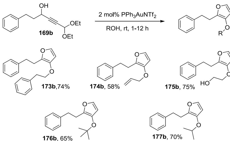
Scheme 101: Synthesis of various 3-alkoxyfurans from propargylic alcohol **169b**
