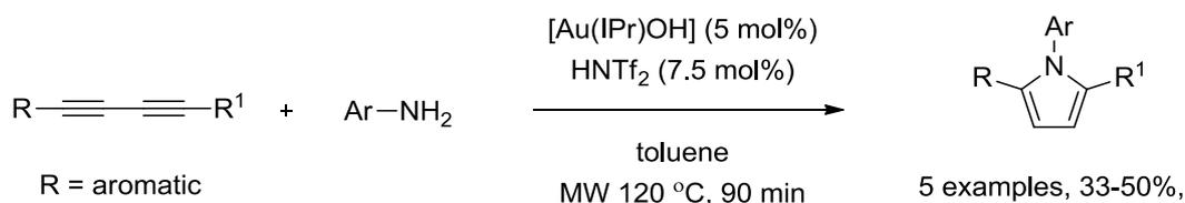
Scheme 25: Au-catalysed pyrrole synthesis <sup>46</sup>
