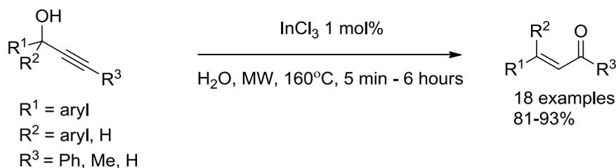
Scheme 62: Microwave assisted  $\text{InCl}_3$  catalysed Meyer-Schuster Rearrangement<sup>112</sup>
