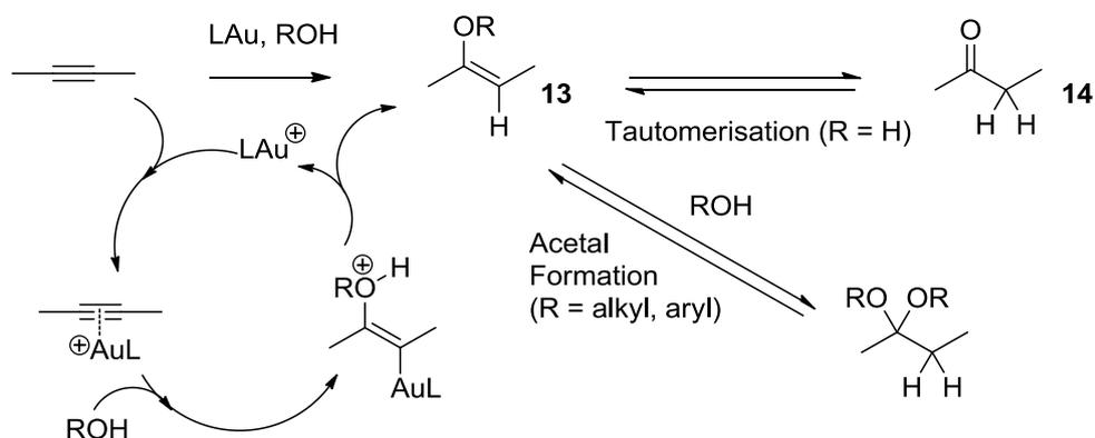
Scheme 8: Alkyne hydration mechanism<sup>16</sup>
