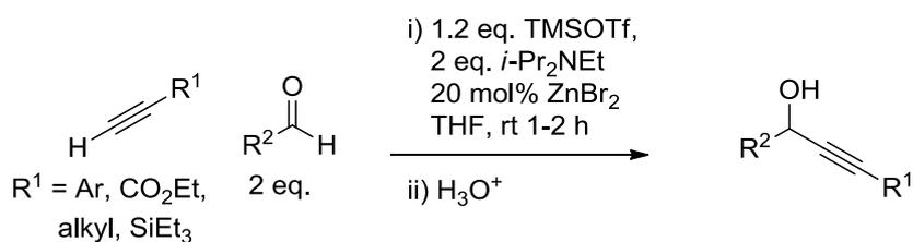
Scheme 36: Zinc catalysed synthesis of propargylic alcohols<sup>68</sup>
