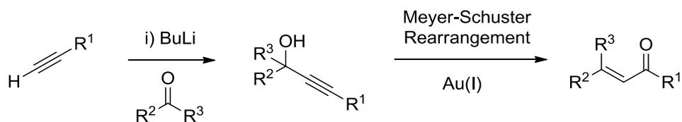
Scheme 48: Meyer-Schuster rearrangement to access  $\alpha,\beta$ -unsaturated carbonyls
