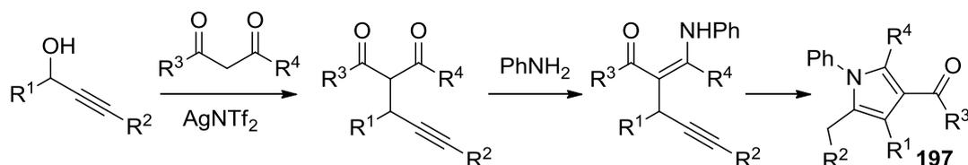
Scheme 118: Pyrrole synthesis through Ag-catalysed substitution
