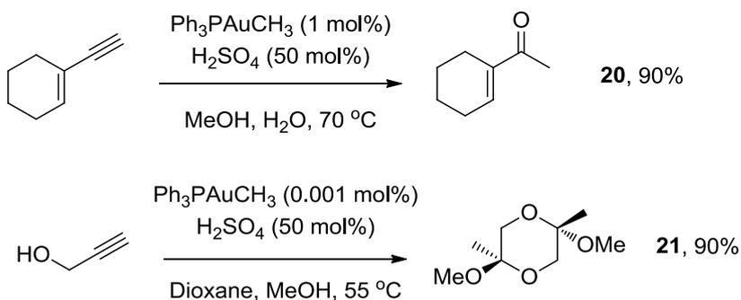
Scheme 11: Low catalyst loadings for hydration of alkyne<sup>30</sup>
