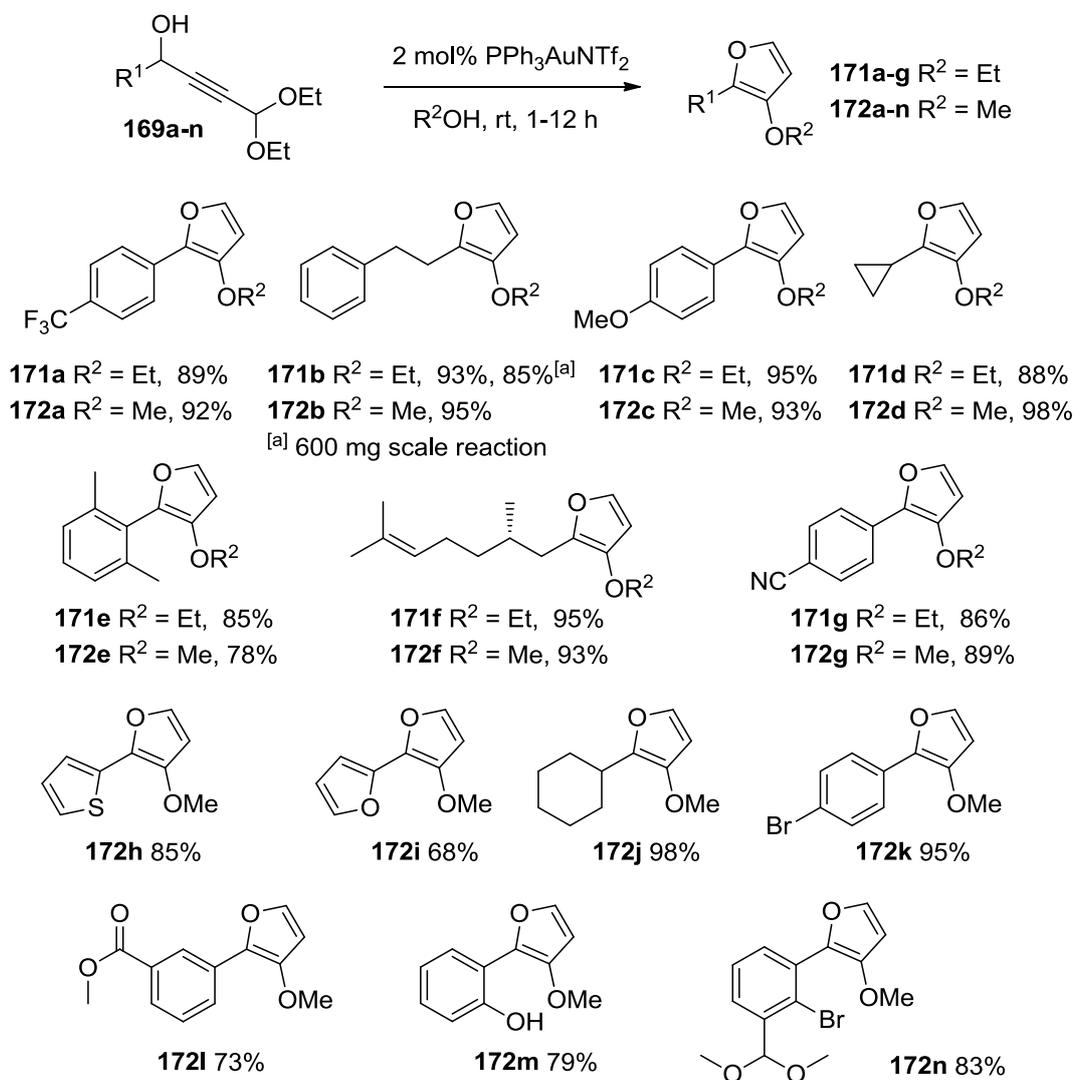
Scheme 100: Au-catalysed synthesis of 3-ethoxyfurans and 3-methoxyfurans
