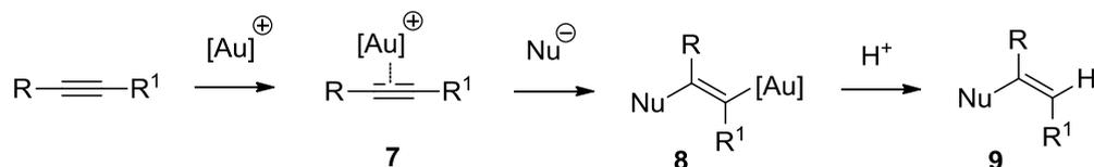
Scheme 6: General reaction scheme for homogeneous Au catalysed activation of alkynes
