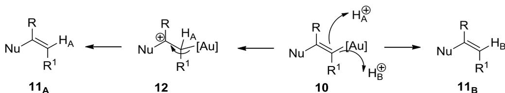
Scheme 7: Possible protodemetalation mechanism routes
