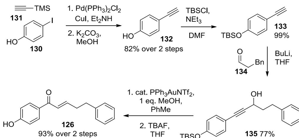
Scheme 74: Synthesis of Daphenone<sup>3</sup>
