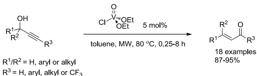
Scheme 63: Vanadate catalysed microwave assisted Meyer-Schuster rearrangement<sup>113</sup>
