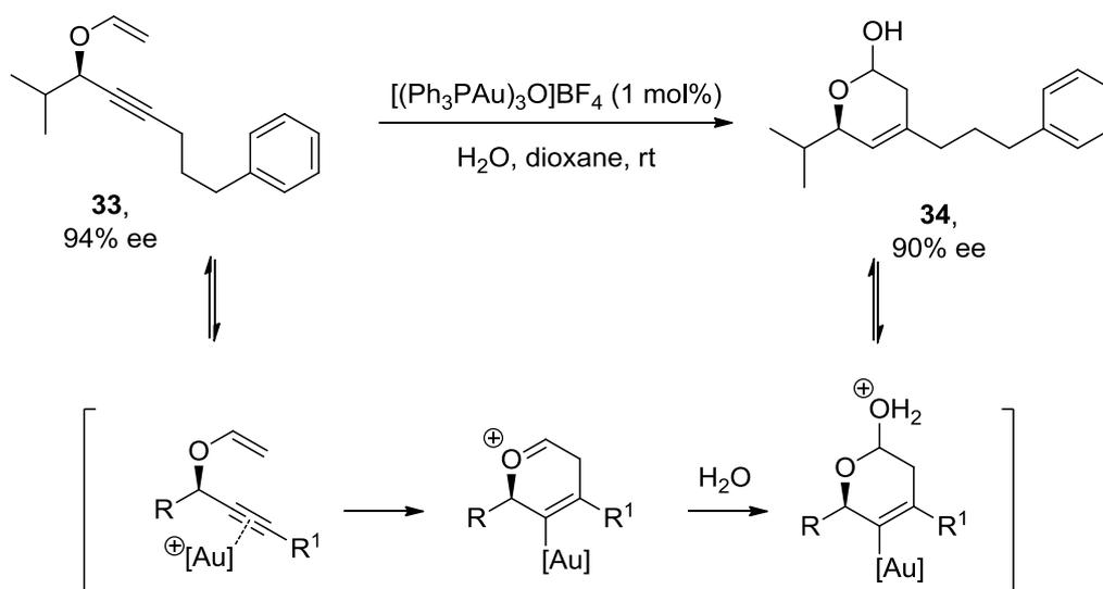
Scheme 20: Au-catalysed cyclisations of enol ethers<sup>42</sup>
