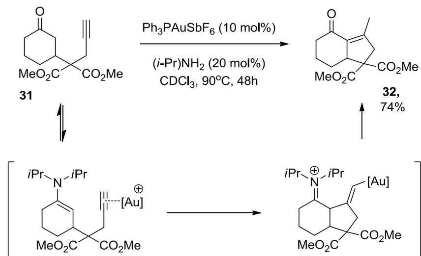
Scheme 19:  $\alpha$ -Functionalisation with alkynes under Au catalysis<sup>41</sup>
