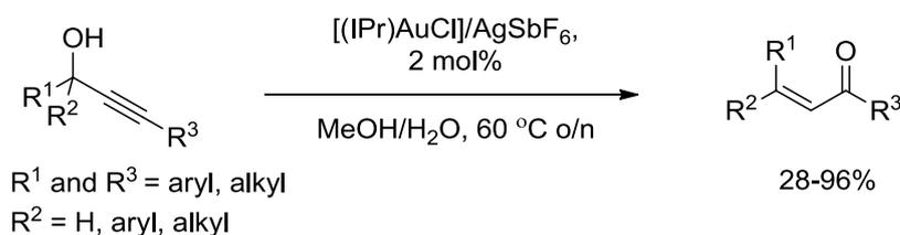
Scheme 53: Au carbene catalysed Meyer-Schuster rearrangement <sup>103</sup>
