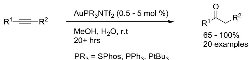
Scheme 13: Room temperature Au catalysed hydration of alkynes
