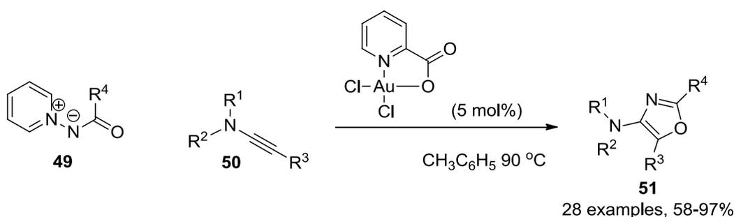
Scheme 27: Au-catalysed synthesis of oxazoles <sup>48</sup>
