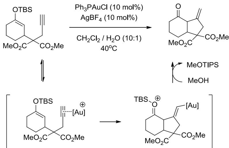
Scheme 21: Au-catalysed cyclisation of silyl enol ethers<sup>43</sup>
