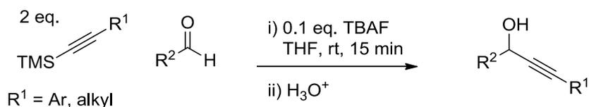
Scheme 37: TBAF mediated synthesis of propargylic alcohols
