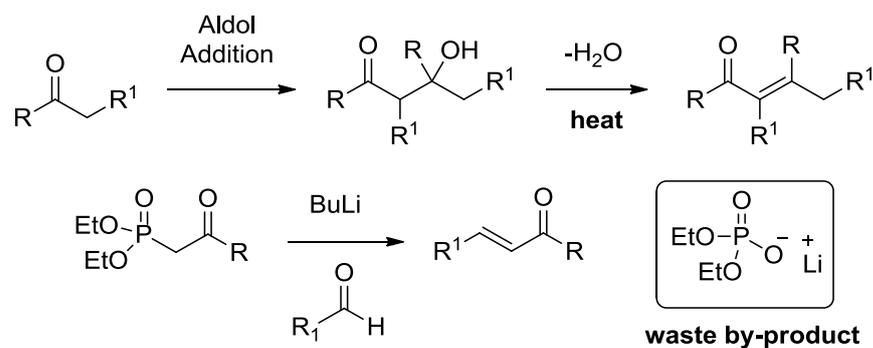
Scheme 47: Traditional methods for access to  $\alpha,\beta$ -unsaturated carbonyls
