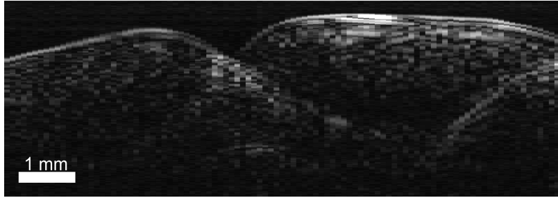
Figure 7. B-mode ultrasound image acquired from the surface of a sheep heart with a 200 \mu\text{m} core optical fiber that was dip coated with the CNT-PDMS composite, and an optical hydrophone. This optical fiber pair was translated in one dimension relative to the tissue surface and the hydrophone signals were concatenated. The scale bar applies to both lateral and depth dimensions.
