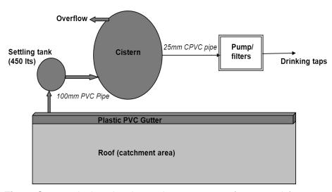
Fig. 1. System design showing main components (not to scale)
