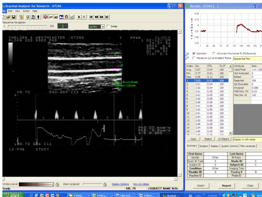
Figure3.2b. Suitable FMD scan for analysis : flat baseline, clean peak and return to baseline
