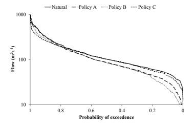
**Fig. 4.** Comparison of the flow duration curves resulting from Policies A, B and C of Fig. 3. Policy C allows around 20% of highest flows to diverge from the natural curve to augment lower flows, maintaining them closer to the natural regime. Policy A achieves the reverse.
