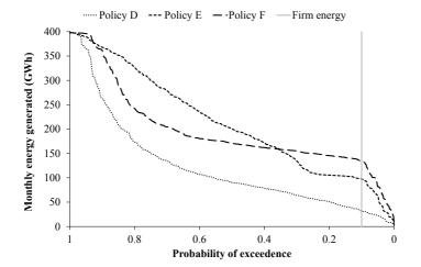
**Fig. 7.** Energy generation implications of the three policies labelled in Fig. 5. Firm energy is the level of generation which can be provided with 90% reliability. Policy F best sustains energy generation to achieve firm energy 326% higher than Policy D and 37% higher than Policy E.
