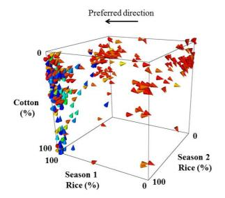
Fig. 11. 3-D (non-trade-off) plot showing the relationship between irrigation scheme selection and agricultural revenue. The solution points are the same as those shown in Fig. 10. High revenues can be achieved with or without the implementation of the cotton scheme. A high proportion of all other schemes must be implemented to achieve maximum revenue however.
