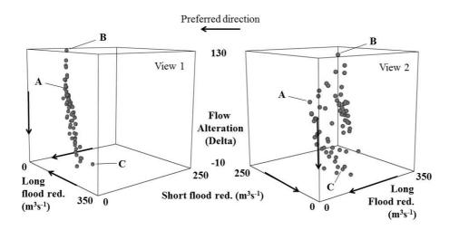
Fig. 3. Two views of the trade-off surface between flow related objectives. Flow regime alteration decreases as flood peaks are reduced allowing lower flows to be maintained closer to the natural regime. Three policies are highlighted and referred to in the text and subsequent figures. A 3-D animation of this plot is available in online Supplement.
