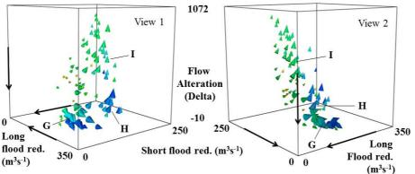
**Fig. 12.** The same trade-off surface as Fig. 10 but restricted to reservoir rules which result in no municipal deficits considering historical data. Such "brushing" of trade-off plots allow stakeholders to focus on system designs that interest them. Three policies are selected for discussion. A 3-D animation of this plot is available in online Supplement.
