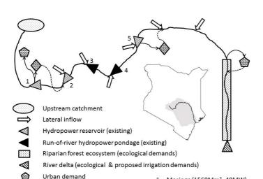
**Fig. 1.** Tana River basin schematic. Inset map shows the location of river and catchment within Kenya.
