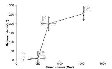
**Fig. 2.** Reservoir release rule (hedging) curves as represented by the IRAS-2010 model. Each patterned pair of opposing arrows represents an optimisation decision variable. Point D is the dead storage of the reservoir. Point A represents the controlled release when the reservoir is full. B and C points can be varied in two dimensions for hedging. In total 5 decision variables define each reservoir's release rule.
