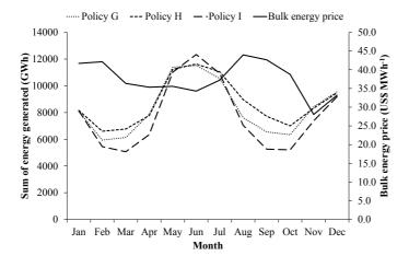
**Fig. 14.** Plot of the total energy generation for each of three selected policies from Fig. 12 alongside the monthly bulk energy price. Higher hydropower revenue (Policy H) is achieved by generating high levels of power in months (August–October) when the bulk energy price is highest.
