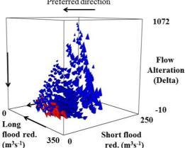
Fig. 9. Trade-off surface of the combined current and proposed demands cases (blue cones show system performance when irrigation schemes can be expanded). Some proposed demands solutions dominate the current demands solutions reducing their representation on the surface. This figure shows how trade-offs achievable by the best system operating rules change once irrigation investments are considered.
