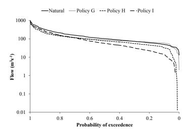
**Fig. 13.** Comparison of the flow duration curves for the three selected operating policies showing the implications of the flow alteration values in Table 1. The Policy G flow regime is closest to natural conditions at both low and mid-range flows, but high flows are sacrificed to increase firm energy. Policies H and I result in the river not reaching the ocean for 1–2% of the time.
