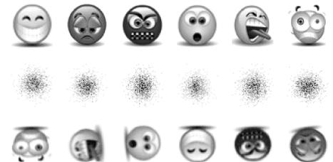
**Figure 3:** Illustration of the ICA-TSP algorithm on the 'smiley' database. Upper row: density function of the sources (using  $10^6$  data points). Middle row: 1,500 samples of the observed mixed signals ( $\mathbf{z}(t)$ ). The ICA-TSP algorithm works on these data. Lower row: Estimated separated sources (recovered up to permutation and orthogonal transformation).
