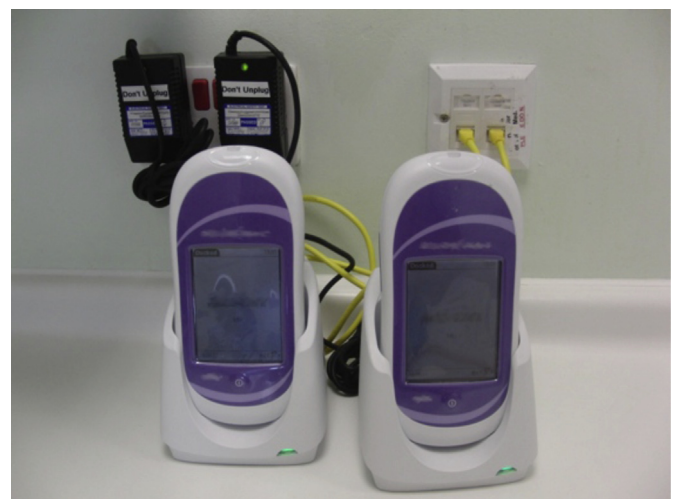
Fig. 1. Blood glucose meters charging in their docking stations. This supplies them with power for recharging and connects them to the network for transferring data.
