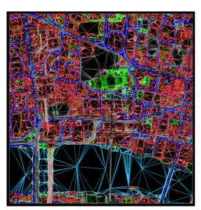
Figure 3 Constrained Delaunay Triangulation
