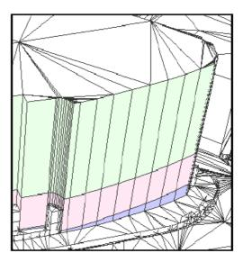
Figure 5 Triangles comprising a building façade
