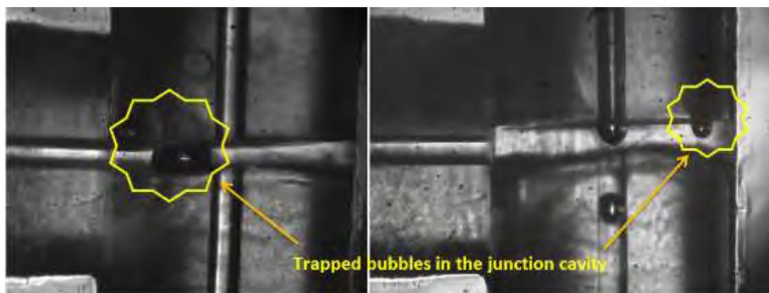
*Figure 4. 12: Existence of trapped bubbles in the junction cavity.*
