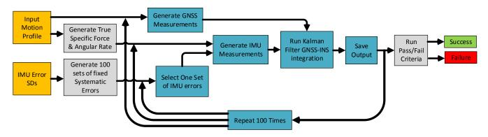
Figure 6. Flow Diagram of the Monte Carlo simulation algorithm. Inputs in yellow and Monte Carlo part in blue.
