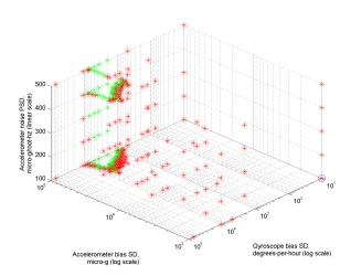
Figure 15. Three dimensional subspace of the search space showing the where the KF fails for different values of accelerometer and gyroscope bias and accelerometer noise with gyroscope noise fixed at 0.01 deg per root hour and both accelerometer and gyroscope unmodelled errors fixed to 'medium' (see Table 3).
