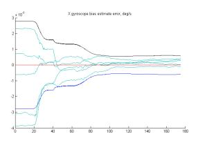
Figure 1. An example of a typical well behaved filter's state estimate error. The filter estimates converge towards zero and their error is well described by the state uncertainty.
