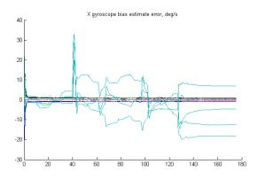
Figure 3. An example of a typical badly behaved filter's state estimate error. The filter estimates do not converge to zero but vary erratically, additionally their variation is much greater than the state uncertainty.
