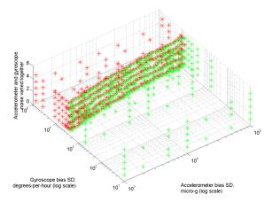
Figure 10. Three dimensional subspace of the search space showing the where the KF fails for different values of accelerometer and gyroscope bias and accelerometer and gyroscope noise varying together and both accelerometer and gyroscope unmodelled errors fixed to 'low' (see Table 3).
