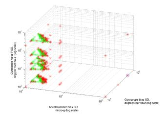
Figure 14. Three dimensional subspace of the search space showing the where the KF fails for different values of accelerometer and gyroscope bias and gyroscope noise with accelerometer noise fixed at  $100 \ \mu g/\sqrt{Hz}$  hour and both accelerometer and gyroscope unmodelled errors fixed to 'low' and 'medium', respectively (see Table 3).
