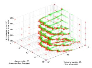
Figure 11. Three dimensional subspace of the search space showing the where the KF fails for different values of accelerometer and gyroscope bias and accelerometer noise with gyroscope noise fixed at 0.01 deg per root hour and both accelerometer and gyroscope unmodelled errors fixed to 'medium' and 'low', respectively (see Table 3).
