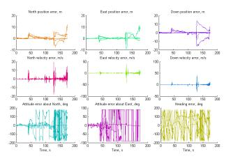
Figure 2. An example of a typical badly behaved filter's estimate errors in its position attitude and velocity solution. Note how the filter starts fairly under control but as soon as the attitude errors about North and East exceed a few tens of degrees (around 30 seconds) then the variation of all the states is becomes extremely erratic.
