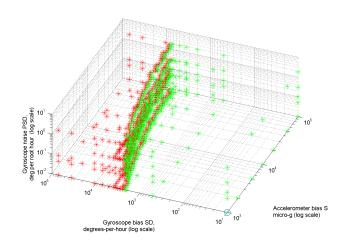
Figure 9. Three dimensional subspace of the search space showing the where the KF fails for different values of accelerometer and gyroscope bias and gyroscope noise with accelerometer noise fixed at 100  $\mu g/\sqrt{Hz}$  hour and both accelerometer and gyroscope unmodelled errors fixed to 'low' (see Table 3).
