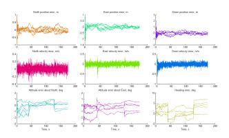
Figure 4. An example of an inconsistently behaved filter's estimate errors in its position attitude and velocity solution. Note how the filter starts fairly under control but as soon as the attitude errors about North and East remain under 2 degrees, making the small angle approximation reasonable, although the heading error is larger.
