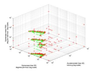
Figure 16. Three dimensional subspace of the search space showing the where the KF fails for different values of accelerometer and gyroscope bias and gyroscope noise with accelerometer noise fixed at 100  $\mu g/\sqrt{Hz}$  hour and both accelerometer and gyroscope unmodelled errors fixed to 'medium' (see Table 3).
