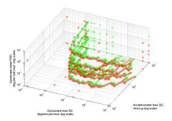
Figure 12. Three dimensional subspace of the search space showing the where the KF fails for different values of accelerometer and gyroscope bias and gyroscope noise with accelerometer noise fixed at  $100 \ \mu g/\sqrt{Hz}$  hour and both accelerometer and gyroscope unmodelled errors fixed to 'medium' and 'low', respectively (see Table 3).
