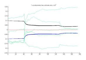
Figure 5. An example of a typical inconsistent filter's state estimate error. Some of the filter estimates converge towards zero but others do not. The spread of estimate errors is not well described by the state uncertainty.
