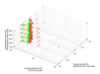
Figure 13. Three dimensional subspace of the search space showing the where the KF fails for different values of accelerometer and gyroscope bias and accelerometer noise with gyroscope noise fixed at 0.01 deg per root hour and both accelerometer and gyroscope unmodelled errors fixed to 'low' and 'medium', respectively (see Table 3).
